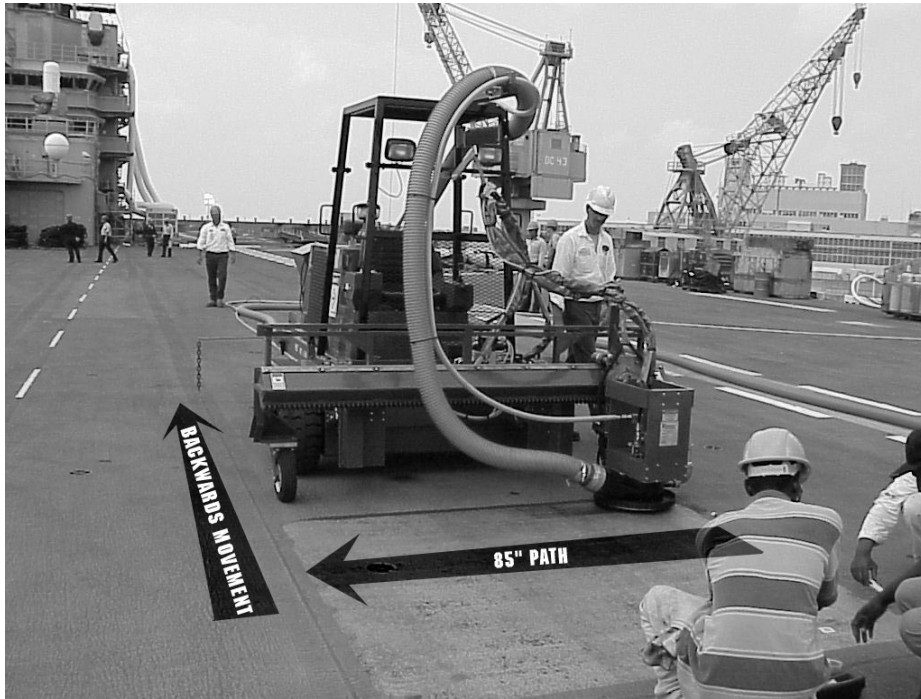
Figure 7. Second generation systems not only traverse backwards, but can index the nozzle array from side to side allowing for up to an 85" cleaning path.
