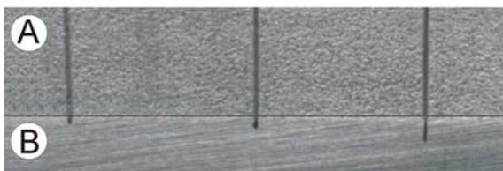
Figure 6. Aluminium and Stainless Steel, Cut with Pure Waterjet at 800 MPa
