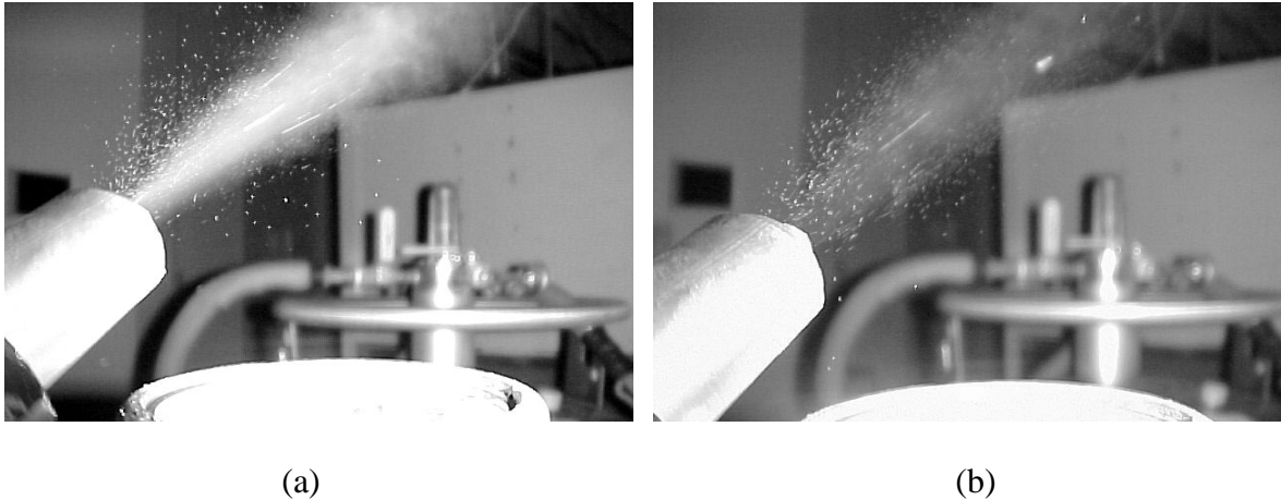
Figure 7. Pictures show the high and low density ice-airjet streams (air pressure = 0.544 MPa, ice particles flow rate is in a range 20g-60g).
