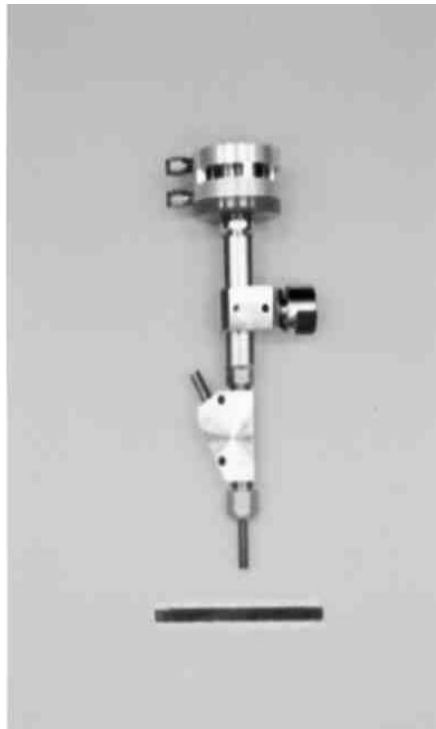
Figure 8. An Air-Valve-Equipped Abrasive-Jet Cutting Nozzle Assembly
