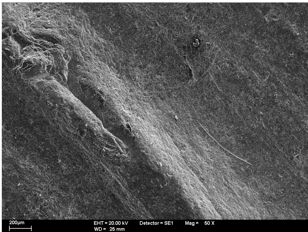
Figure 14. SEM images of Capão Bonito Red Granite cut by abrasive waterjet. On top, smooth zone. On bottom, rough zone.
