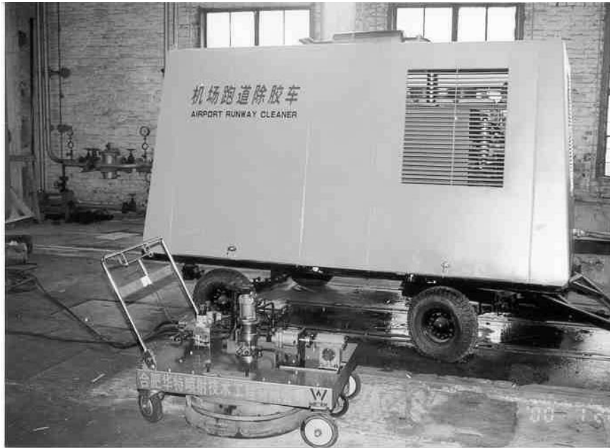
Figure 3. Equipment for Glue Removal on Airport Runway
