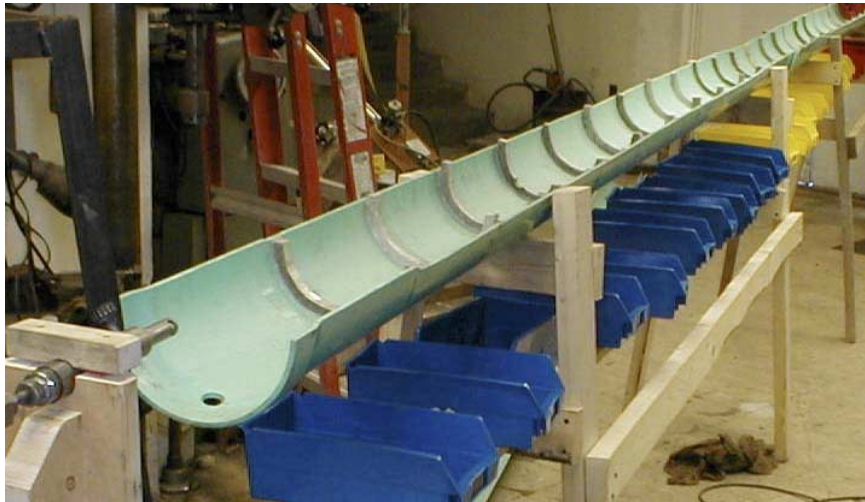
Figure 1. Test arrangement to determine the throw and size reduction of abrasive through an AWJ nozzle.
