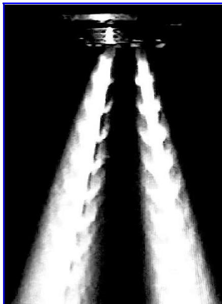
Figure 8. Typical appearance of the forced pulsed waterjet from a dual-orifice nozzle.
