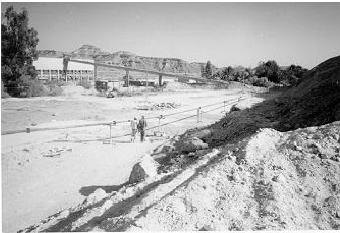
Figure 15. Water-phosphate slurry flow through pipeline on the surface to the classifier.
