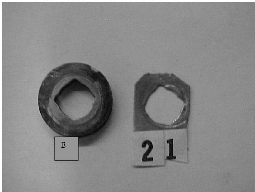
Figure 8. Piercing of stainless steel sample (21) at non round opening in the base (B). Notice geometrical similarity between the hole in the sample in the opening in the base.
