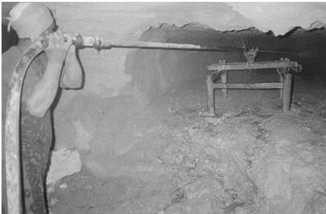
Figure 3. The high-pressure monitor, cutting the phosphate seam.
