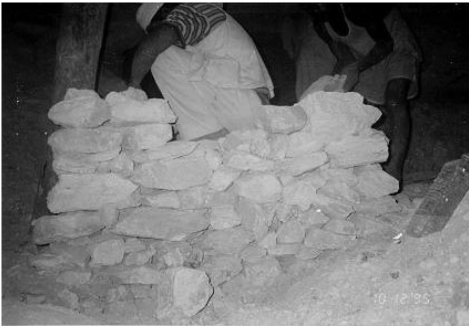
Figure 7. Roof support by building rock pillars.
