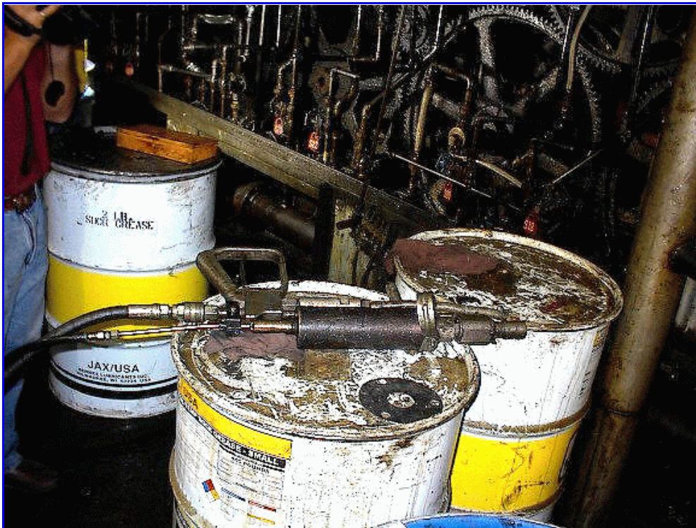
Fig. 7. A general view of the shortened gun fitted with a non-rotating single orifice nozzle.
