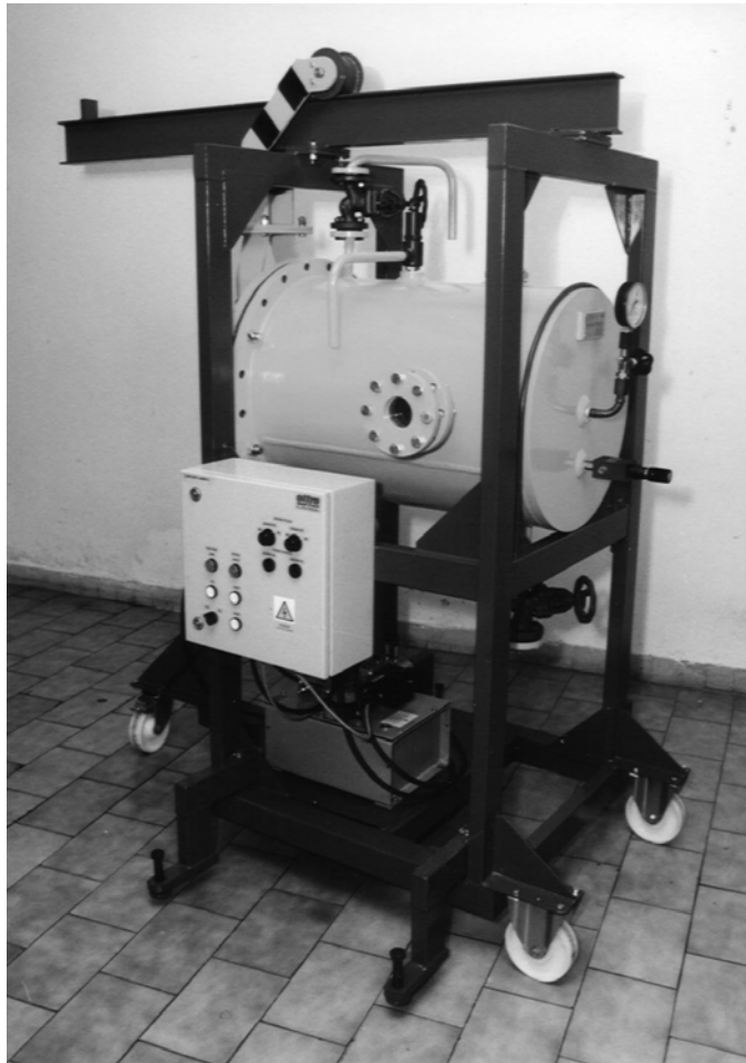
Figure 1. The mobile pressure vessel for testing of water jet in pressurized surrounding water up to 5 MPa.
