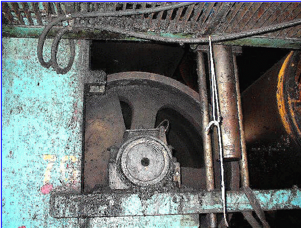
Fig. 5. A general view of the roll showing the bearing at the centre covered with grease.
