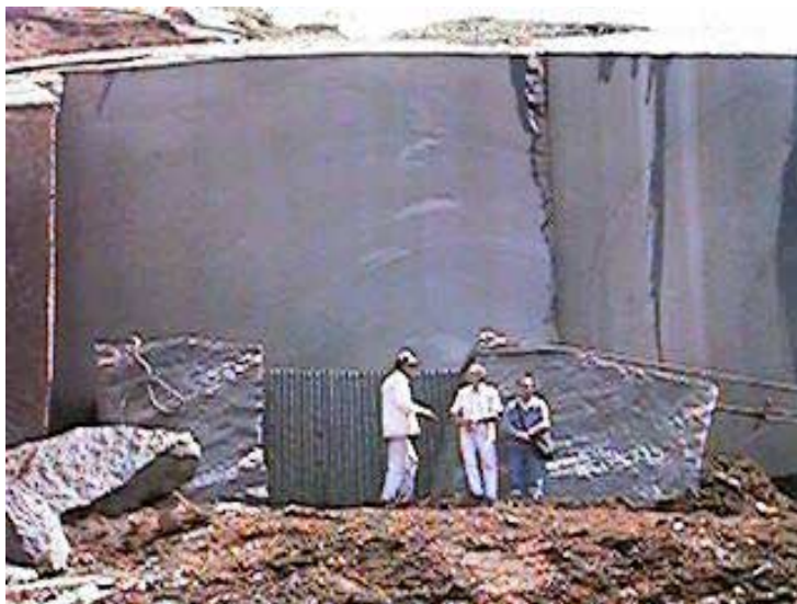
Figure 4. Diamond wire block winning at Piracaia Black Granite Quarry
