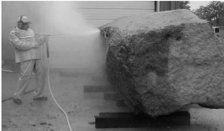
Figure 8. Distressing the blocks with a hand-held lance.
