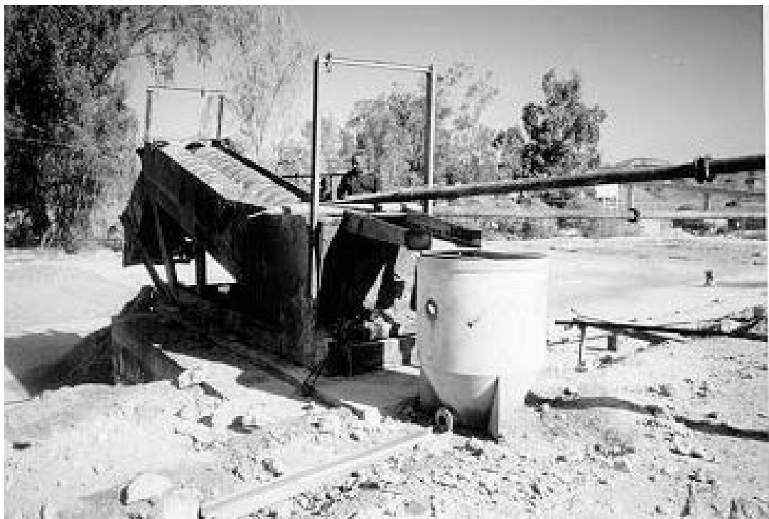
Figure 16. Water-phosphate slurry flow through pipeline to the classifier, water and clay are directed to nearby valley. Some of this water is used to irrigate nearby small farm.
