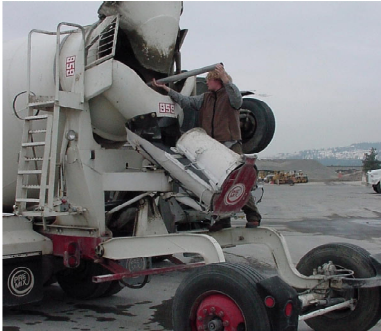
Figure 3. View showing limited access to tank interior.
