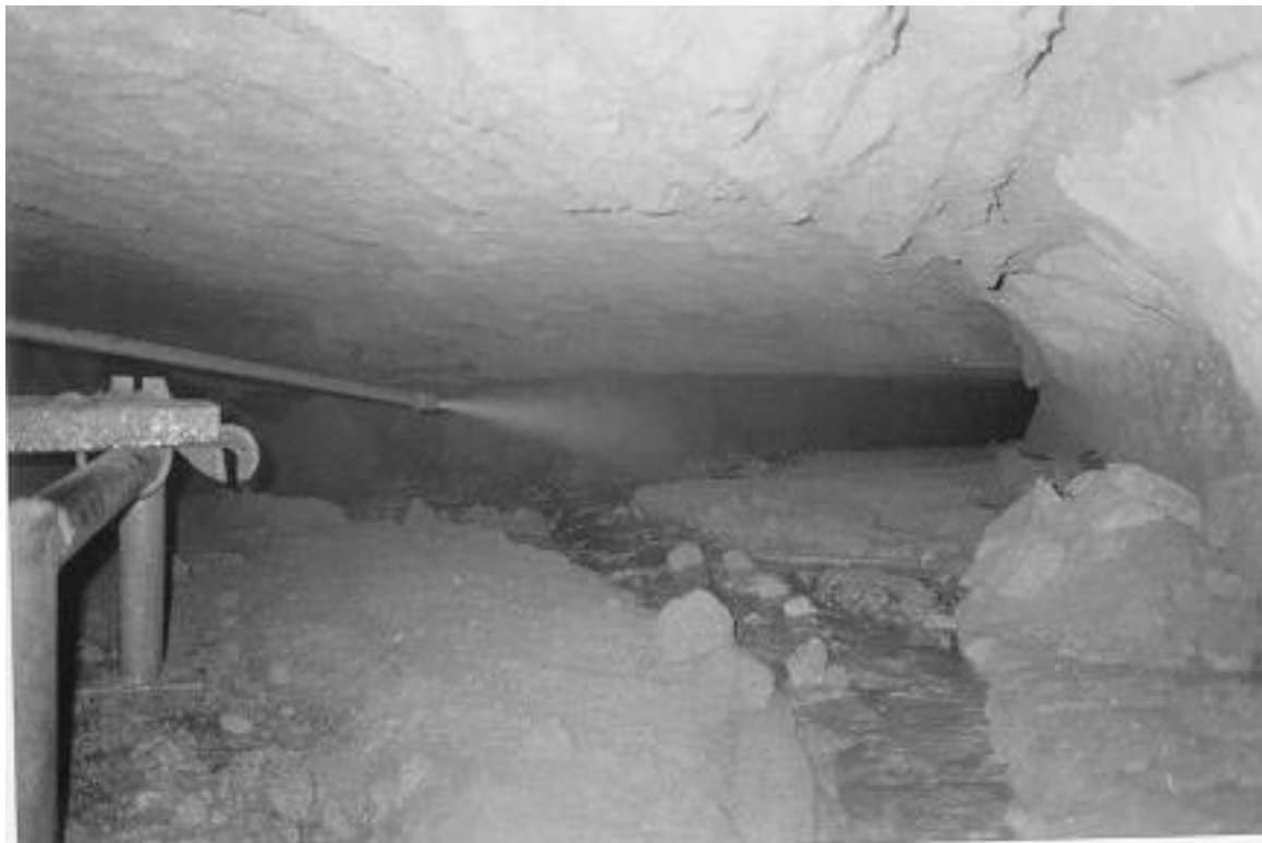
Figure 10. The High Pressure Monitor, cutting the phosphate seam, water-phosphate slurry flow through dug channels in the mine floor.
