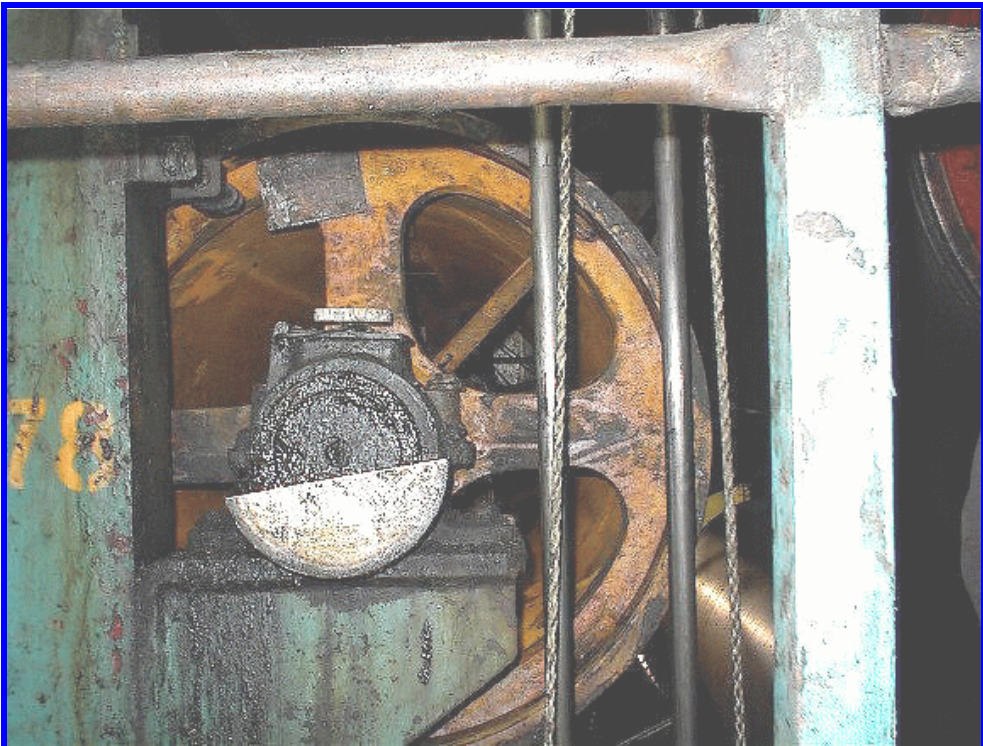
Fig. 6. A general view of the head of the roll after cleaning with the forced pulsed waterjet (rust is believed to be acceptable).
