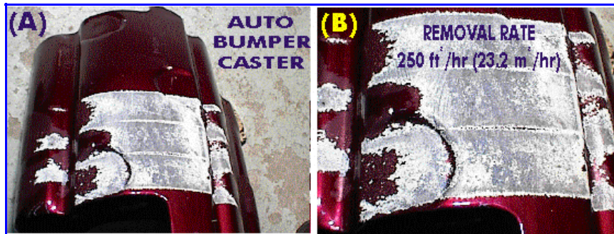
Figure 11. Multiple layers (~ 14 layers) of paint removed with the rotating forced pulsed waterjet from the auto bumper casters. (B) Closed-up of the surface finish.
