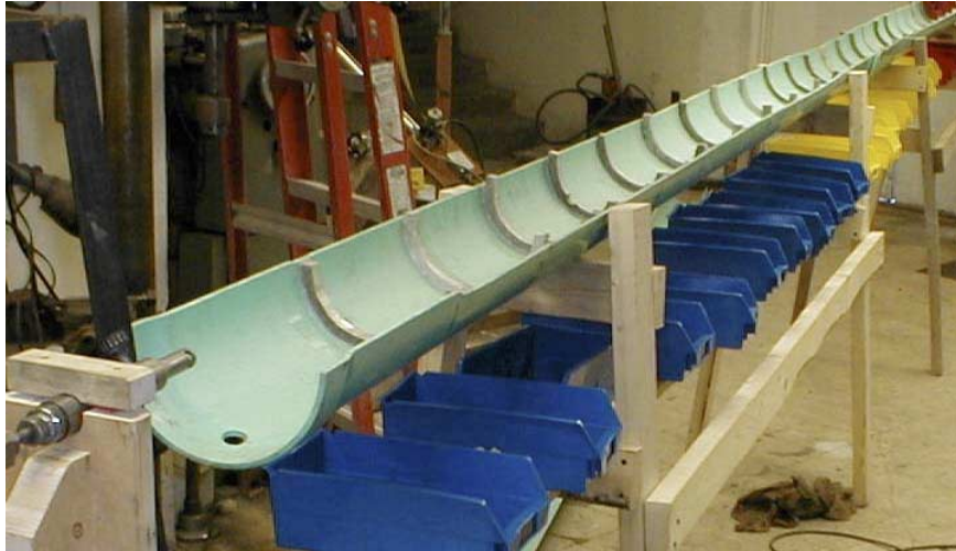
Figure 2. Particle analysis test setup – in a test additional segments were attached to the tube, which extended beyond the door, and a covering tube enclosed the stream.
