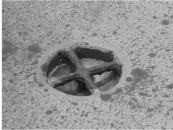
Figure 3. Tie downs or "padeyes" provide areas where steel shot can escape onto the deck of the carrier.
