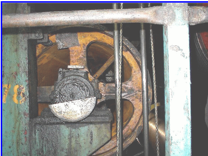
Figure 16. A general view of the head of the roll after cleaning with the forced pulsed waterjet (rust is believed to be acceptable).
