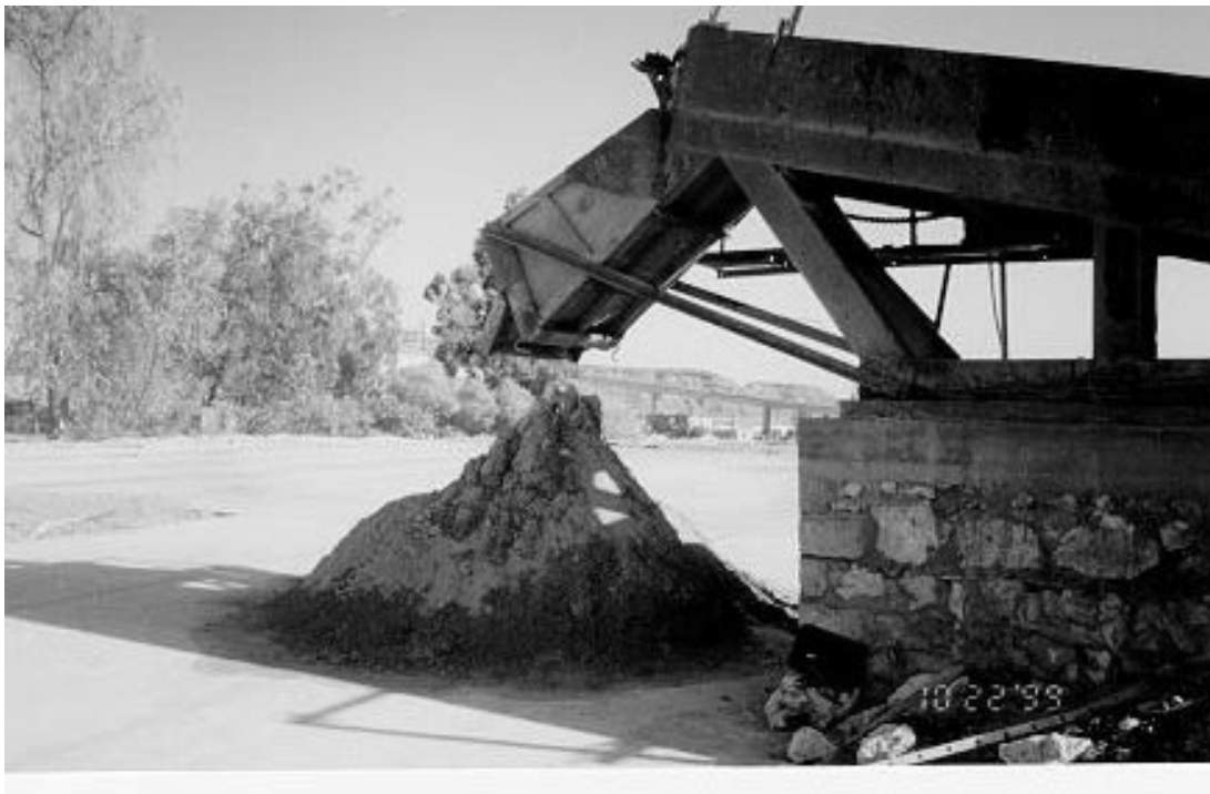
Figure 17. The phosphate concentrate produced from the spiral classifier.
