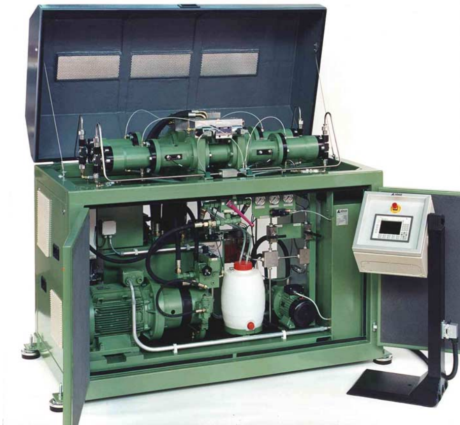
Figure 1. Autofrettage Pump Adapted for Waterjet Cutting at 800 MPa.
