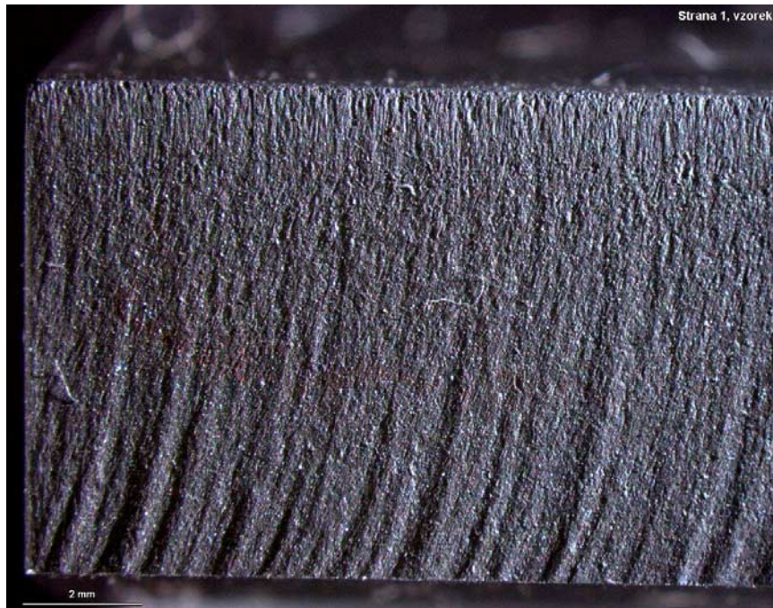
Figure 2. The character of the walls made by abrasive water jet in the slot.
