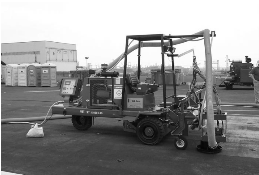
Figure 6. Second generation non-skid removal systems combine the advantages of the original systems with new features that improve productivity.
