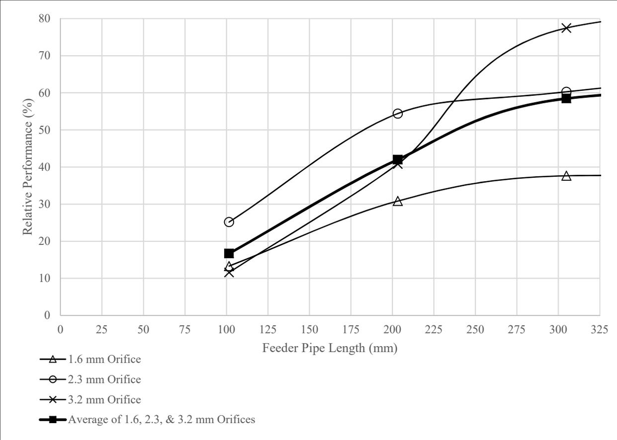
**Figure 6.** Curtailed view of Figure 5. Relative performance of increasing feeder tube length for various orifice sizes, Ø20.7 mm ID feeder pipe. Note stabilization of performance with increasing length.
