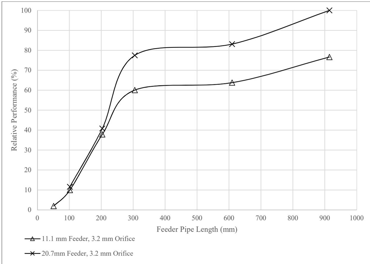
**Figure 7.** Relative performance of 3.2 mm (.125 in) orifices in 11.1 mm (.438 in) and 20.7 mm (.815 in) feeder pipes of varying length. Performance relative to 3.2 mm (.125 in) orifice with Ø20.7 mm by 914 mm (Ø.815 in x 36 in) feeder pipe. Note similar performance with short feeder pipes and improved performance with a larger diameter feeder pipe as the length increases.
