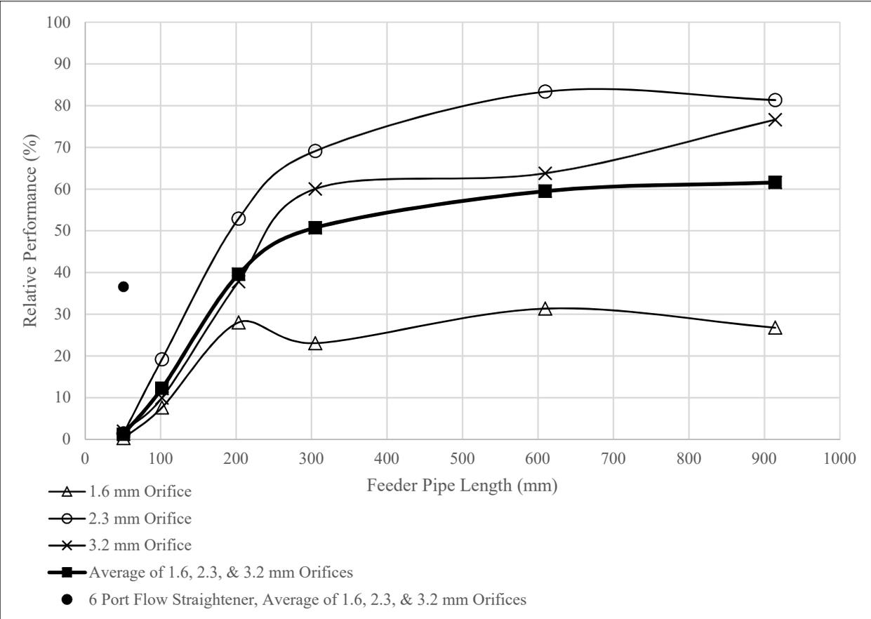
**Figure 3.** Relative performance of increasing feeder tube length for various orifice sizes, Ø11.1 mm ID feeder pipe. Performance relative to 3.2 mm (.125 in) orifice with Ø20.7 mm by 914 mm (Ø.815 in x 36 in) feeder pipe. Note stabilization of performance with increasing length as well as increased performance with a flow straightener.
