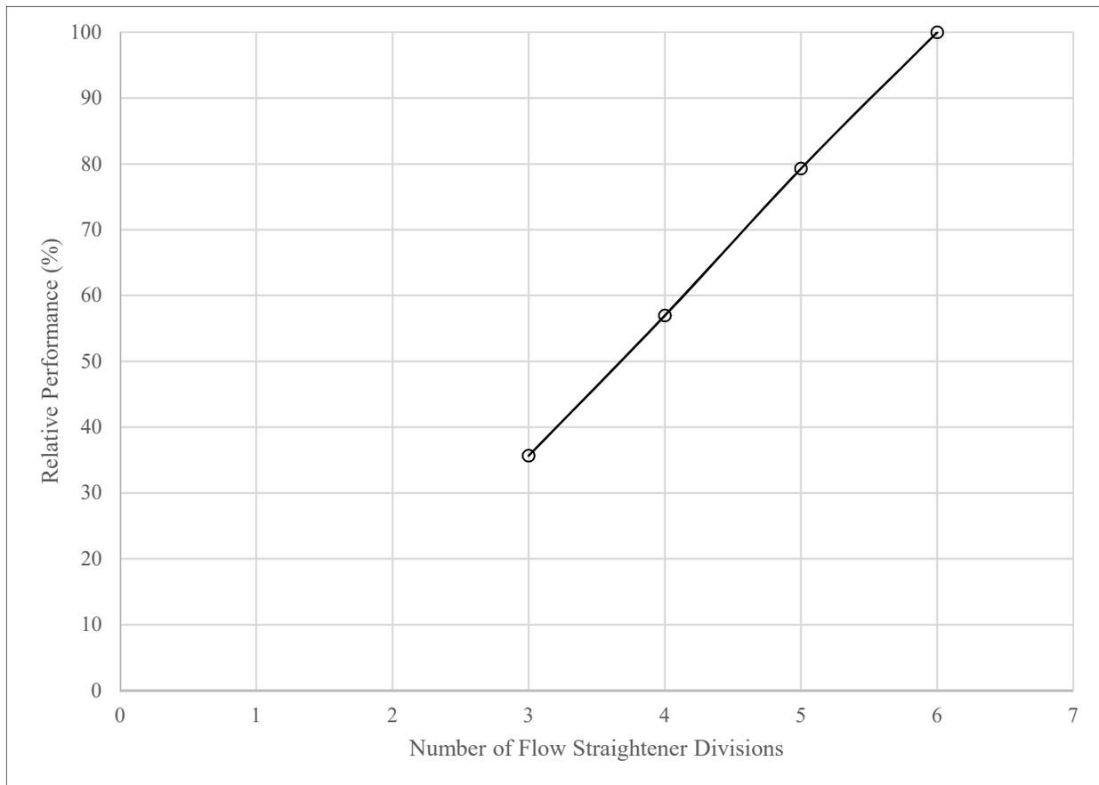
**Figure 8.** Relative performance of number of flow straightener divisions. Performance relative to average of 1.6, 2.3, and 3.2 mm (.063, .090, .125 in) orifices with  $\text{\O}11.1$  mm by 51 mm ( $\text{\O}.438$  in x 2 in) feeder pipe. Note the trend of increasing performance with increasing divisions as well as the slope of the line suggesting that the trend may continue past six divisions.
