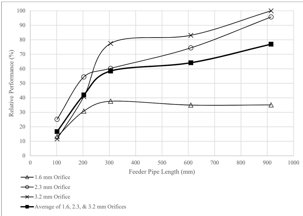
**Figure 5.** Relative performance of increasing feeder tube length for various orifice sizes, Ø20.7 mm ID feeder pipe. Performance relative to 3.2 mm (.125 in) orifice with Ø20.7 mm by 914 mm (Ø.815 in x 36 in) feeder pipe. Note stabilization of performance with increasing length.
