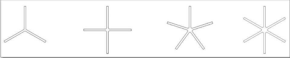
**Figure 2.** Flow straightener cross sections showing styles with 3, 4, 5, and 6 divisions.
