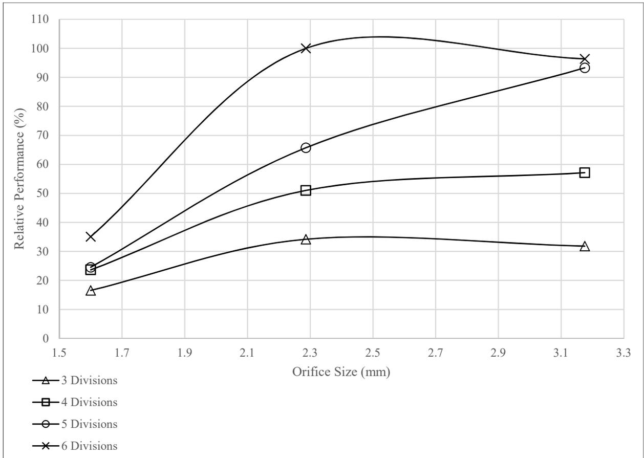
**Figure 9.** Relative performance of increasing the number of flow straightener divisions vs nozzle size. Performance relative to a 2.3 mm (.090 in) orifice with a six-division flow straightener installed in a  $\text{\O}11.1$  mm by 51 mm ( $\text{\O}.438$  in x 2 in) feeder pipe. Note that the optimal orifice size may be larger than 3.2 mm (.125 in) for the flow straighteners with four and five divisions.
