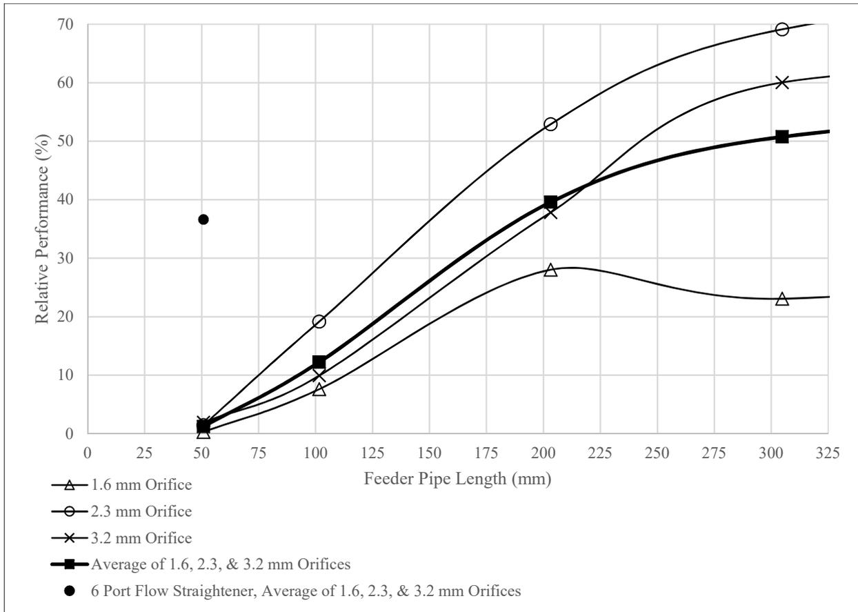
**Figure 4.** Curtailed view of Figure 3. Relative performance of increasing feeder tube length for various orifice sizes, Ø11.1 mm ID feeder pipe. Performance relative to 3.2 mm (.125 in) orifice with Ø20.7 mm by 914 mm (Ø.815 in x 36 in) feeder pipe. Note stabilization of performance with increasing length as well as increased performance with a flow straightener.
