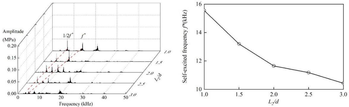
**Figure.5** Characteristics changing as a function of  $L_2/d$ .(a) Spectrum of the pressure signal spectrum at point 2; (b) self-excited frequency evolution as increasing of  $L_2/d$ .
