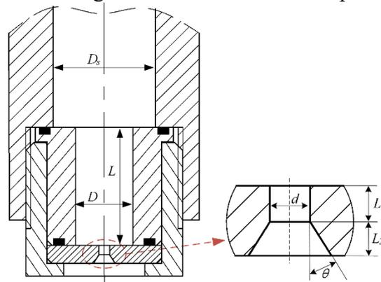
Figure 2. Schematic diagram of the organ-pipe nozzle and lip geometry.(a) Organ-pipe nozzle; (b) Enlarge of the nozzle lip
