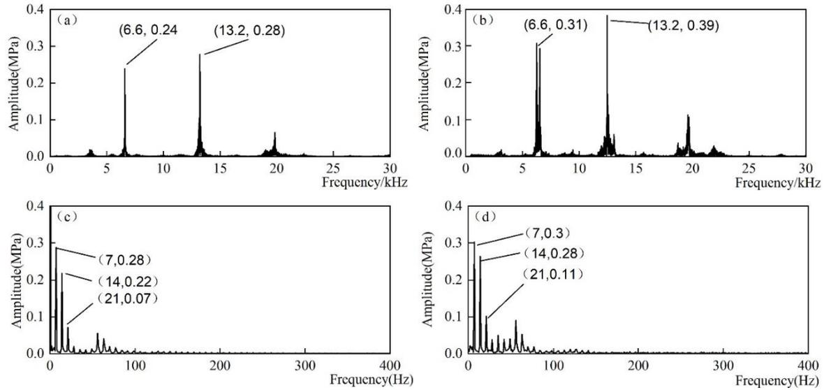
**Figure.4** Spectrum of the pressure signal: (a) spectrum at point 2; (b) spectrum at point 4; (c) low frequency spectrum at point 2; (d) spectrum at point 1
