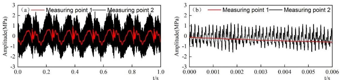
**Figure 3.** (a) Time-domain waveform of the pressure signal and (b) the locally amplified time-domain waveform
