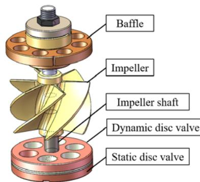
Figure.1 Novel Disc-type Pulsed Water Jet Generator
