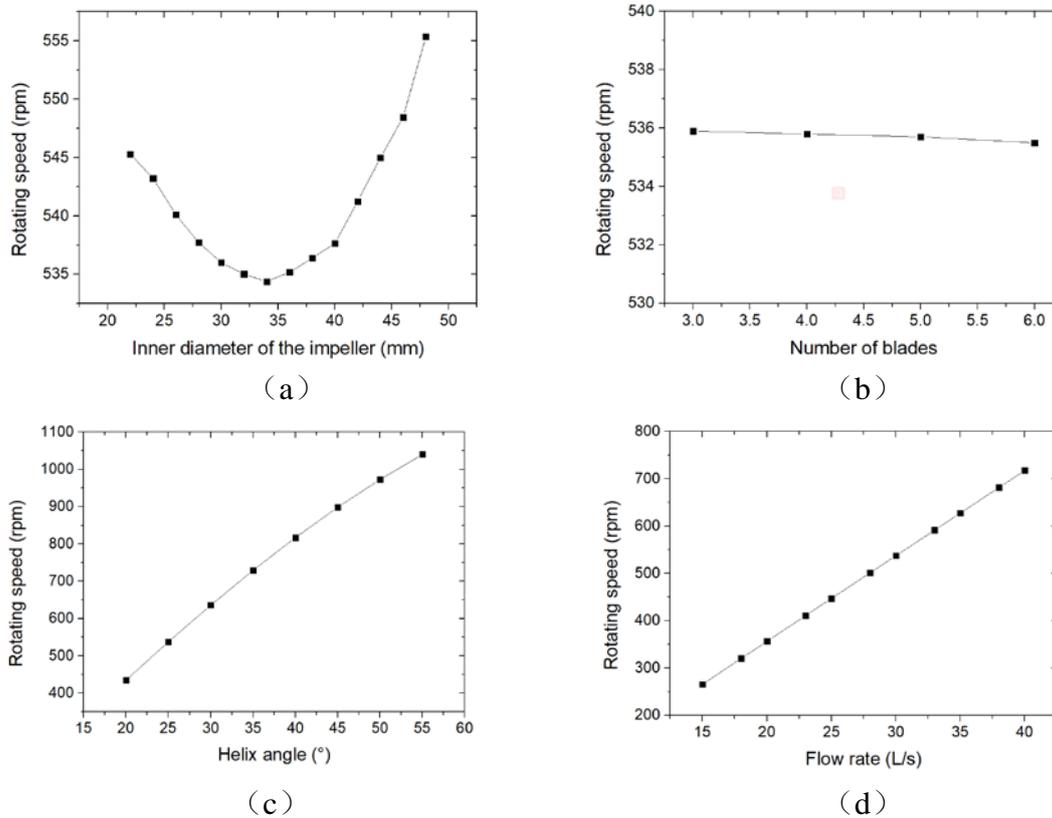
Figure.4 The Rotating Speed of the Impeller Varies with (a) Inner Diameter, (b) the Number of Blades, (c) the Helix Angle and (d) the Flow Rate of Drilling Fluid
