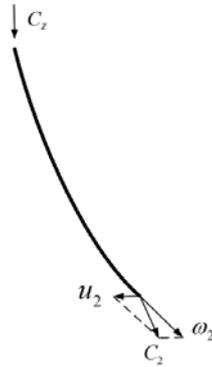
Figure 3. Diagram of Impeller Inlet and Outlet Velocity
