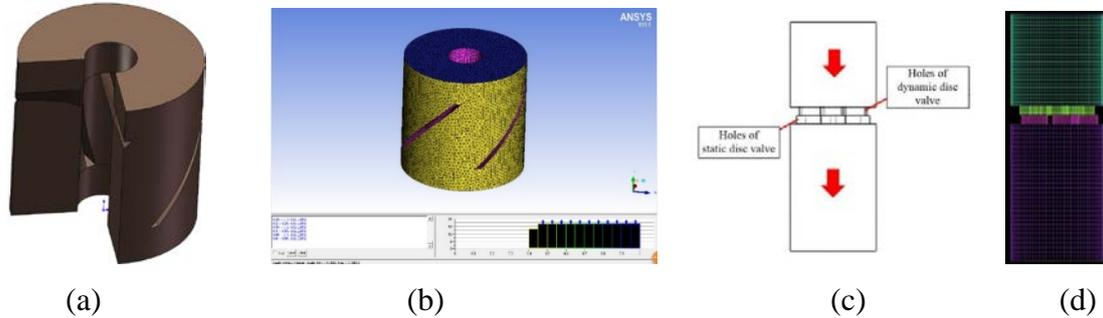
Figure.5 Geometric Model and Structure Division of Impeller and Pulse Generating Mechanism
