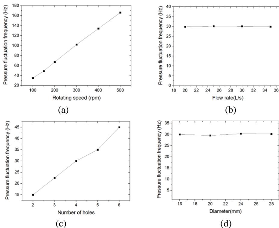
Figure.13 Pressure Fluctuation Frequency Changes with (a) Rotating Speed, (b)Flow Rate, (c) Number of Holes, (d) Diameter of Holes
