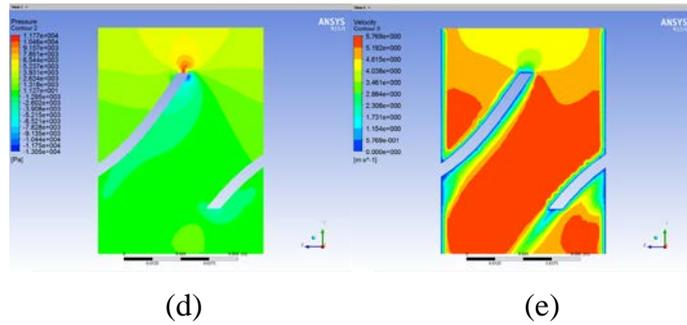
Figure.6 Pressure and Velocity Distributions Near Impeller(a) Three-dimensional Pressure Distribution, (b) Flow Diagram, (c) Surface Pressure Distribution of Impeller, (d) Side View of Pressure Distribution, and (e) Side View of Velocity Distribution
