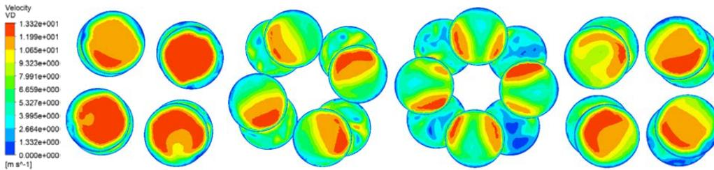
Figure.10 Velocity Distribution of the Pulse Generation Mechanism
