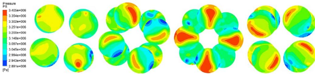
Figure.9 Pressure Distribution of the Pulse Generation Mechanism
