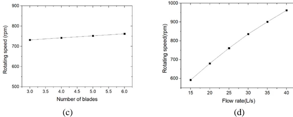
Figure.8 Rotating Speed Changes with (a) Helix Angle of the Blade,(b) Inner Diameter of Impeller,(c) Number of Blades,(d) Flow Rate of Drilling Fluid
