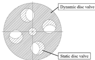
Figure.2 Mechanism Diagram of Pulsed Jet Flow
