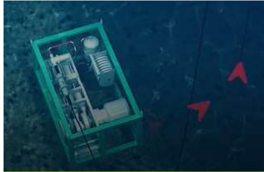
Figure 1. Ultra high pressure sea water submarine pump unit
