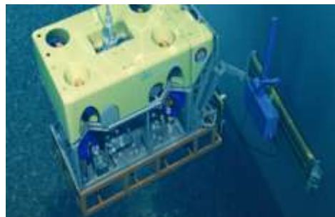
Figure 2. Ultra high pressure water cutting device cooperated with ROV
