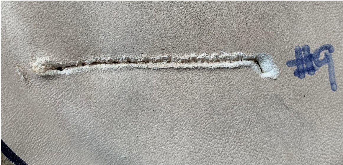
Figure 4. Cut from a Traverse of Skin Simulant by 0.8 mm (.031 in) Orifice at 13.8 MPa and 4.5 lpm (2000 psi and 1.2 gpm)
