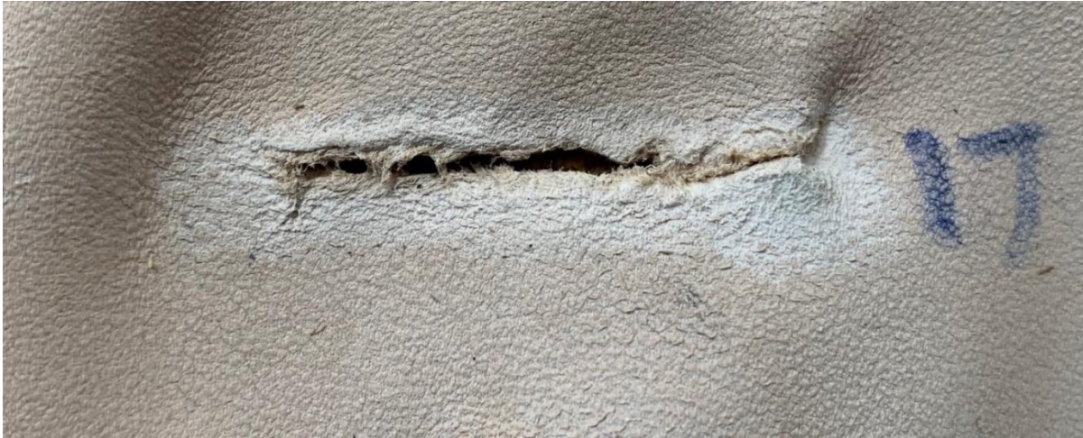
Figure 5. Cut from a Traverse of Skin Simulant by 3.0 mm (.118 in) Orifice at 10.3 MPa and 55 lpm (1500 psi and 14.5 gpm)
