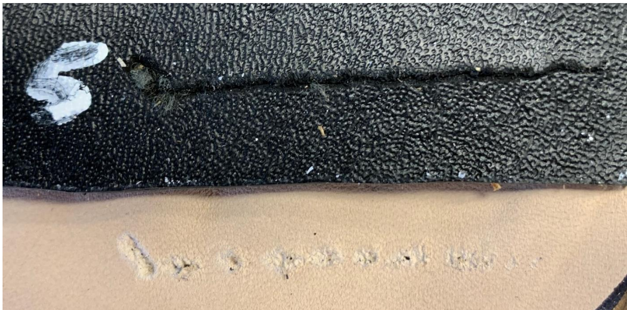
Figure 6. Penetration of Skin Simulant Placed Behind Rubber Boot Material
