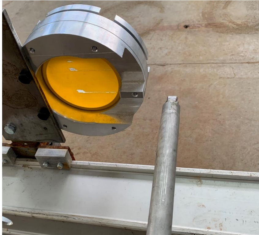
Figure 1. Sample Holder and Traversing Nozzle Lance Test Arrangement
