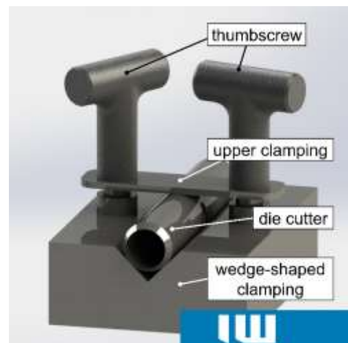
Figure 3. Mechanical fixation device with die cutter.
