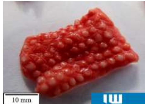
Figure 6. Nubs on the tissue surface caused by the suction through the perforated sheet
