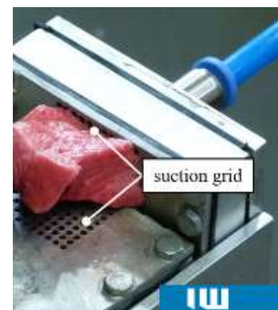
Figure 5. Fixation of tissue specimens with low-pressure suction
