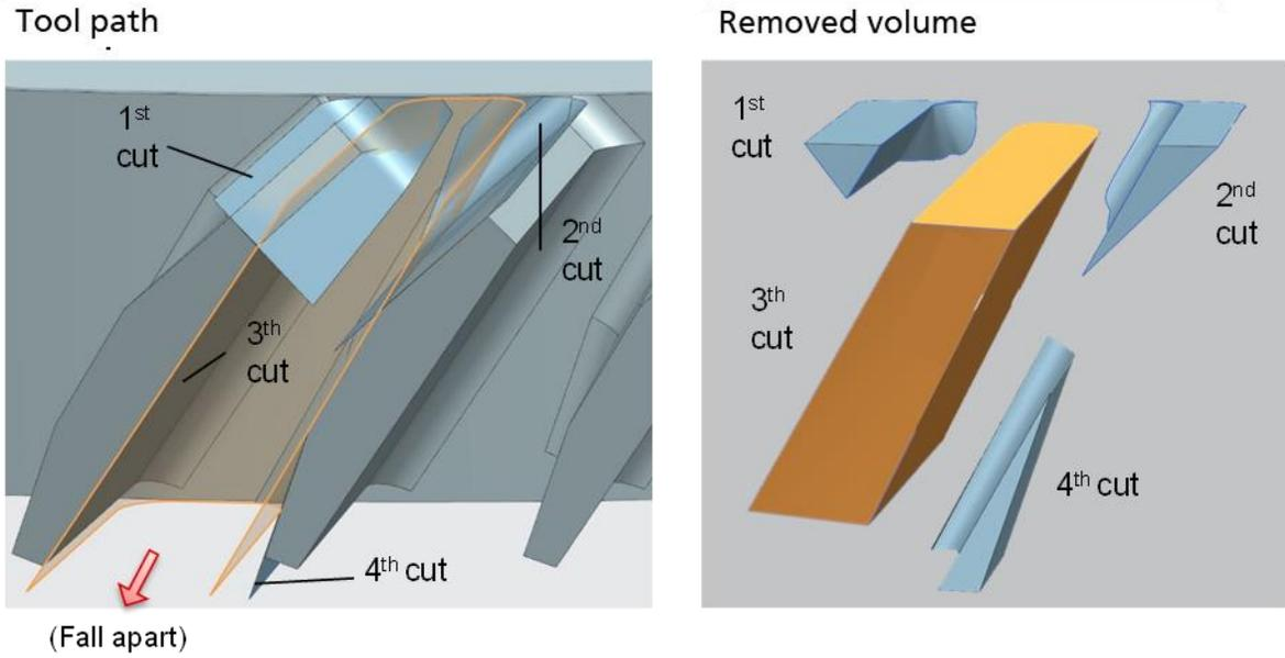
**Figure 5:** Tool path design and cut out pieces
