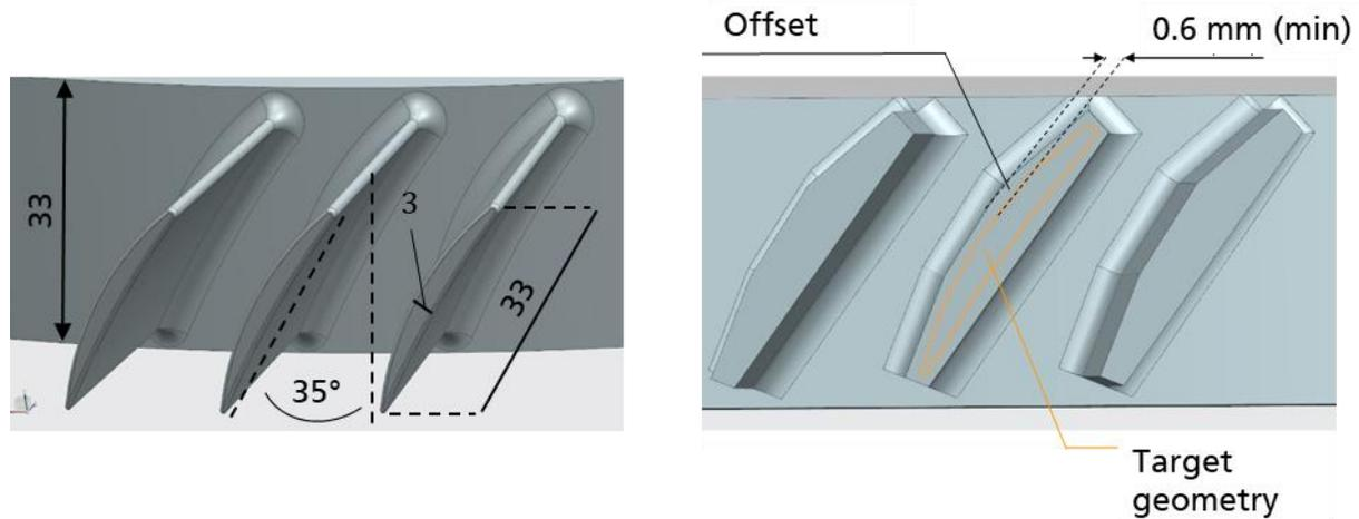
**Figure 4:** Geometry offset added to the contour of the BLISK CAD model
