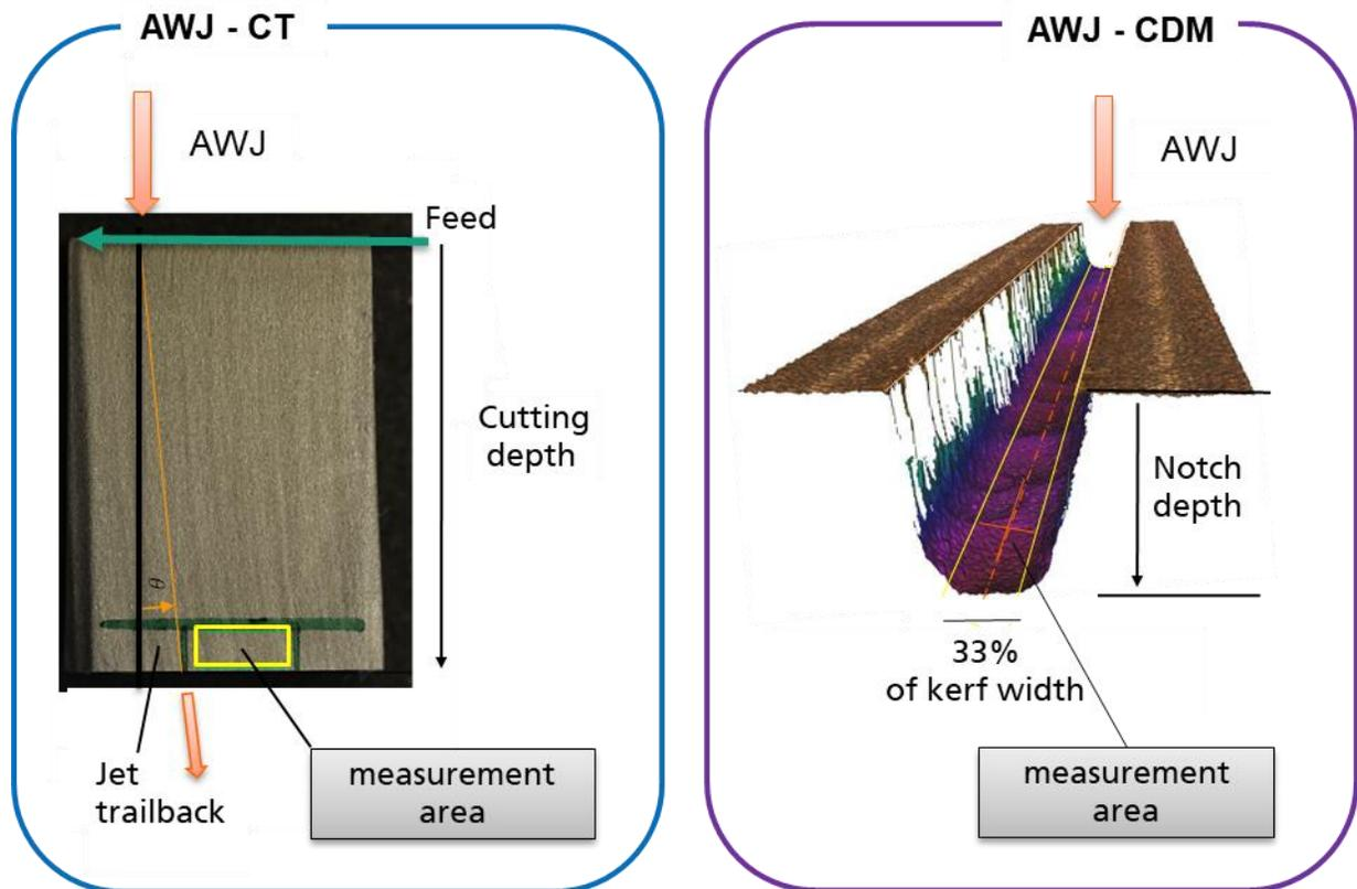
**Figure 3:** Analysis scheme of the test pieces
