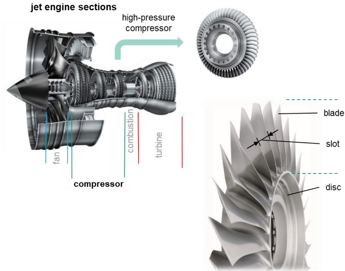
**Figure 1:** BLISK part within a modern jet engine compressor section
