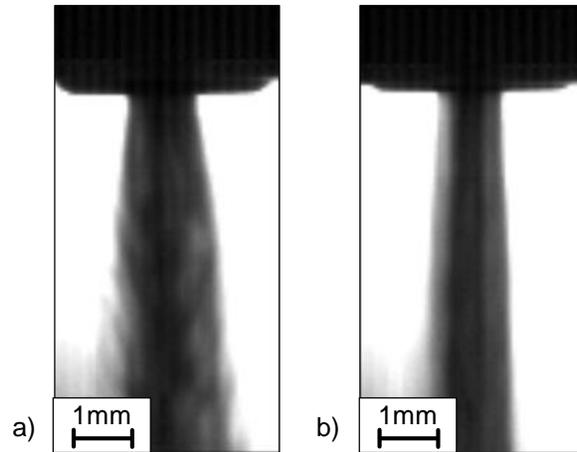
**Figure 6.** CO<sub>2</sub> jet with  $d_D = 0.1$  mm at; a)  $p_0 = 100$  MPa; b)  $p_0 = 300$  MPa [8]
