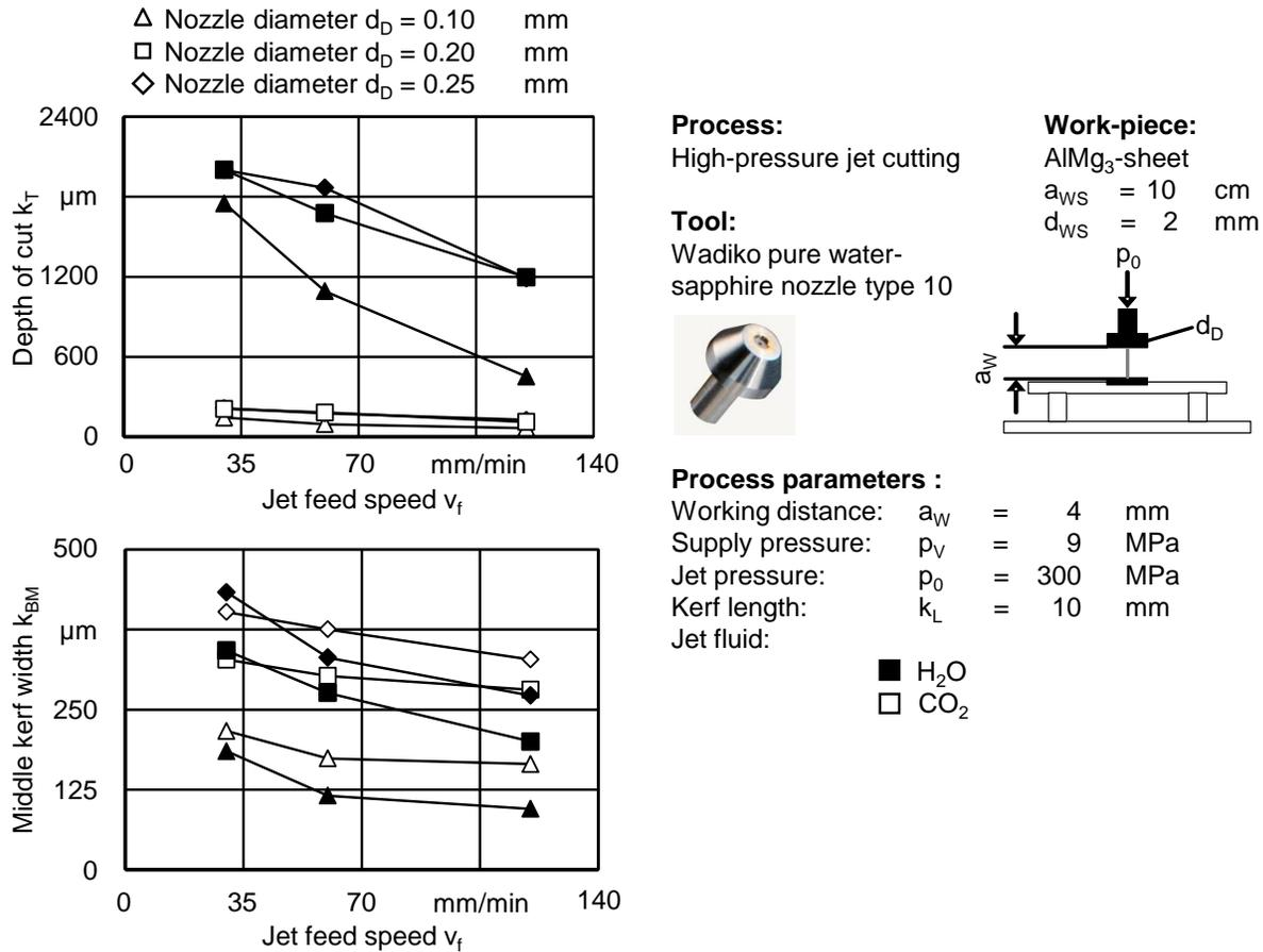
**Figure 3.** Depth of cut  $k_T$  und middle kerf width  $K_{BM}$  depending on jet feed speed  $v_f$
