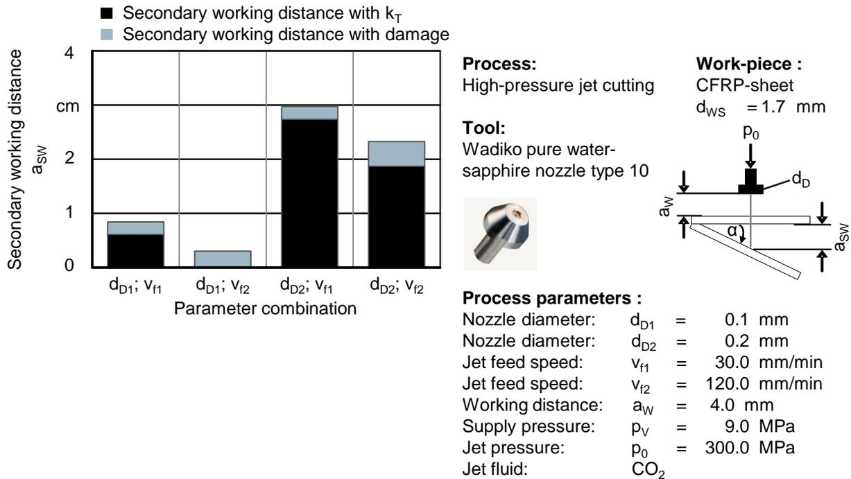
**Figure 7.** Secondary working distance  $a_{SW}$  with a depth of cut  $k_T$  and damage of the workpiece
