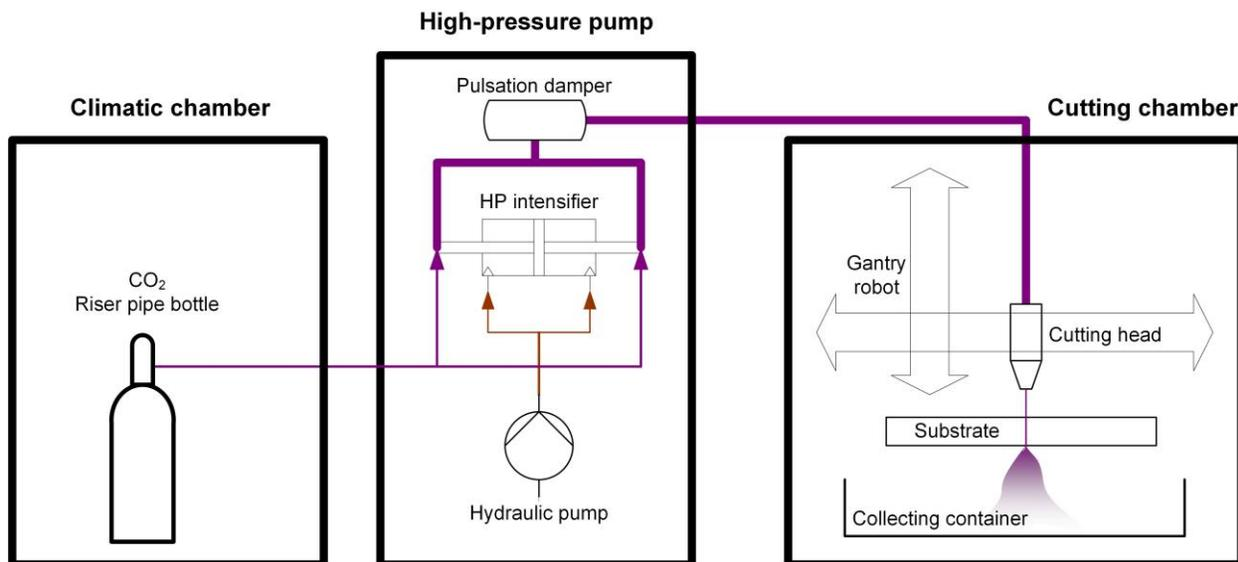
**Figure 1.** Schematic sketch of the high-pressure liquid CO<sub>2</sub> jet cutting system
