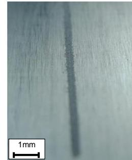
CO<sub>2</sub>-jet cutting of AlMg<sub>3</sub>
