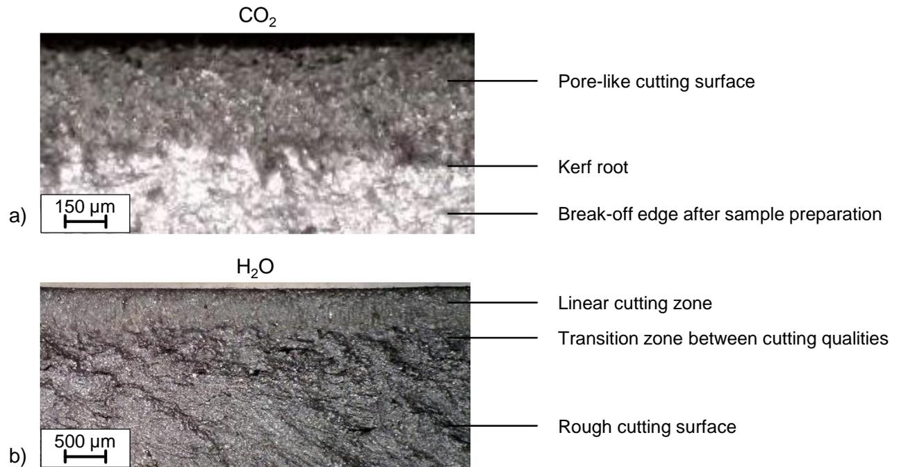
**Figure 4.** Lateral cutting surface for  $p_0 = 300$  MPa,  $v_f = 30$  mm/min,  $a_w = 4$  mm; a) CO<sub>2</sub> jet,  $d_D = 0.12$  mm; b) H<sub>2</sub>O jets,  $d_D = 0.25$  mm
