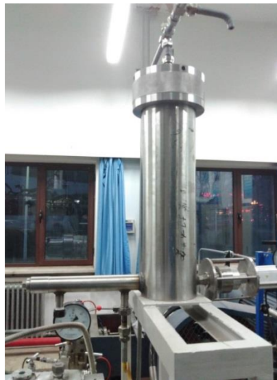
Fig. 2 Abrasive feeding facility
