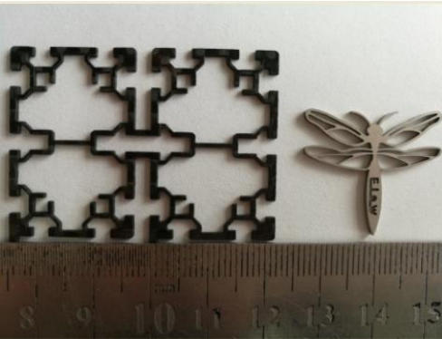
Figure4. Micro Water Cutting Processing
