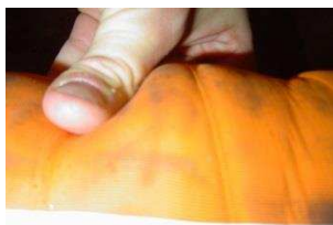
blisters, soft or bulging hose
