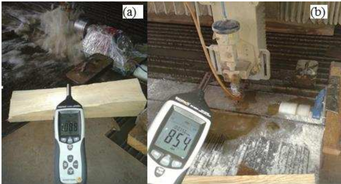
Figure 6. (a) Turning with abrasive water jet over the water level, (b) turning with abrasive water jet under the water level.
