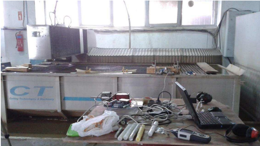
Figure 2. The water jet machining machine used in the experiment.
