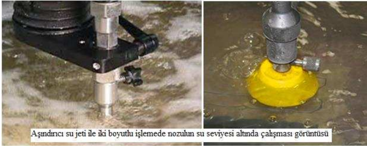
Figure 1. Two-dimensional cutting process below the water level of abrasive water jet,
