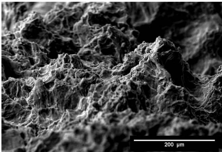
**Figure 2.** SEM image (200X) showing PWJ roughened surface free of grit contamination.
