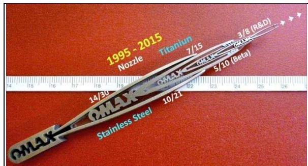
Figure 13. Progress in AWJ micromachining
