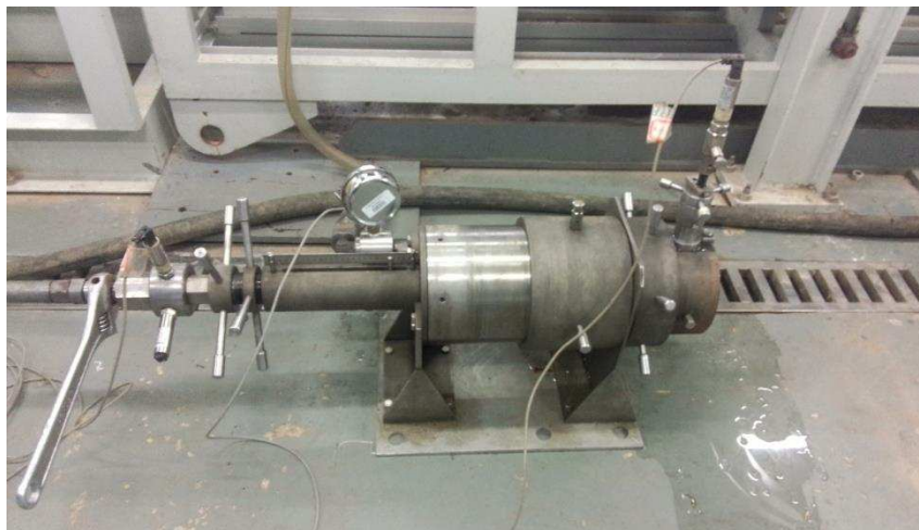
Figure 2. Photo of High Pressure Water Jet Simulator
