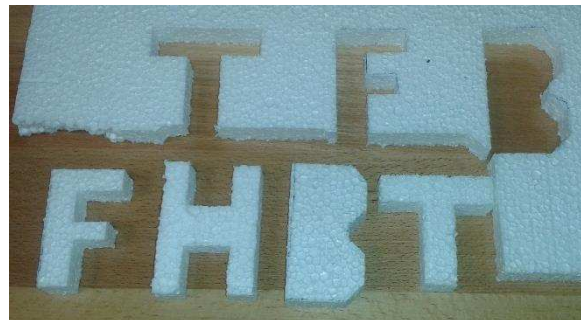
Figure 7. The image of the sample letters cut from styrofoam with the water jet.
