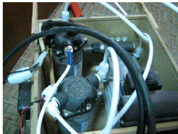
Figure 2. The pump unit is derived from pressure washer.
