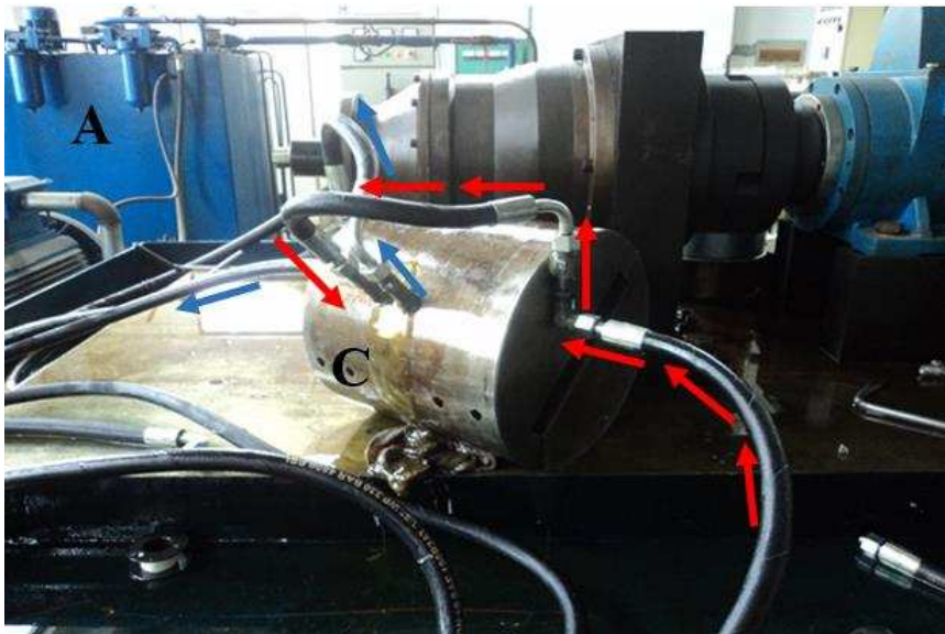
Figure 13. Hemispherical Vane Motor Testing Prototype Picture
