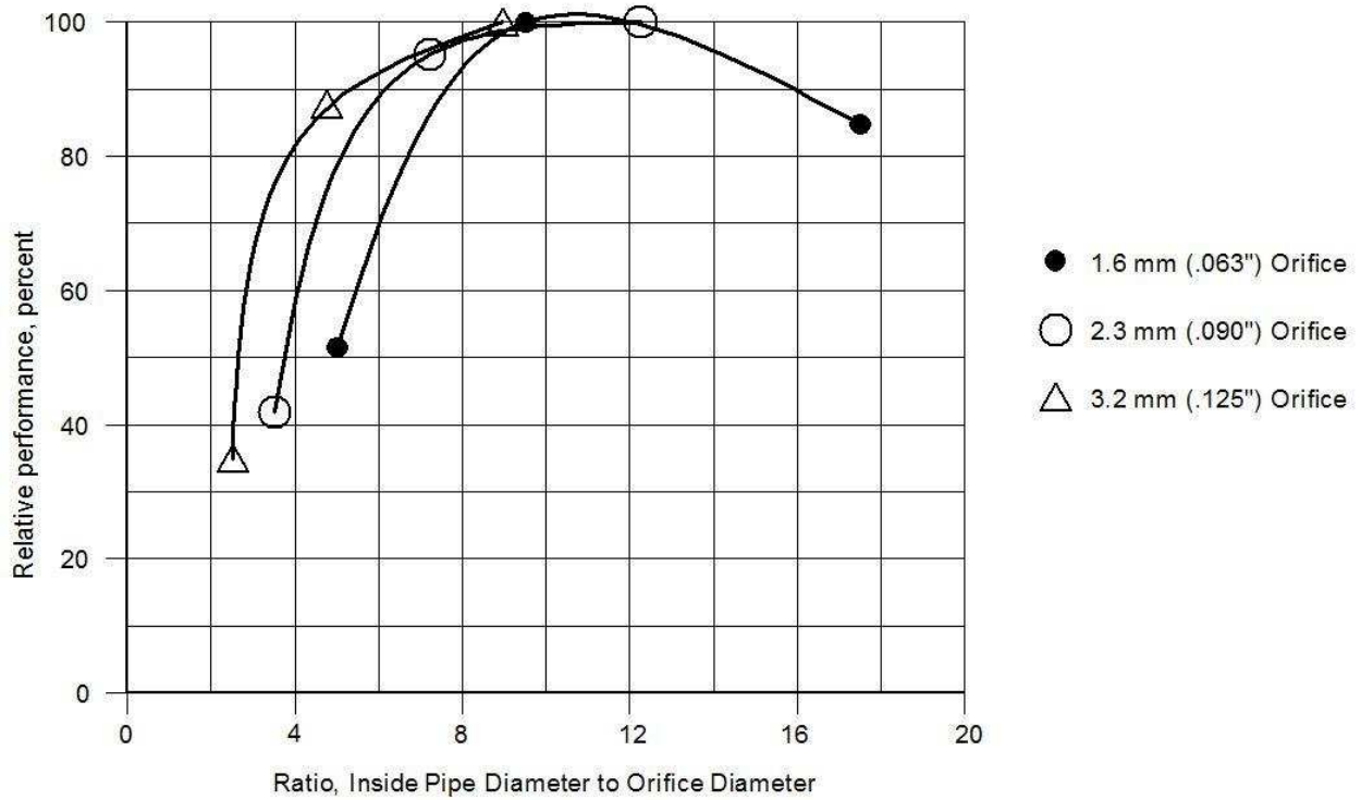
Relative Performance at a Feeder Tube Length to Inside Diameter Ratio of 12:1 Figure 11.
