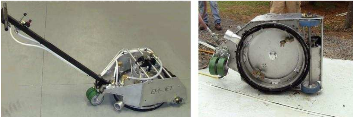
Figure 5. Epi-jet prototyper equipment (Left), View of underside showing nozzle carriers (Right)
