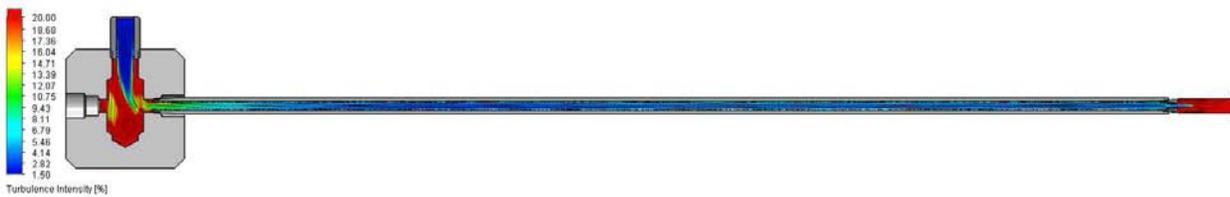
**Figure 17:** Turbulence Intensity with an Overlay of Velocity Streamlines - Showing 7.9mm (.312") Inside Diameter, 914mm (36") Long Tube with 3.2mm (.125") Orifice
