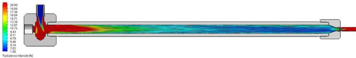
**Figure 16:** Turbulence Intensity with an Overlay of Velocity Streamlines - Showing 27.9mm (1.1") Inside Diameter, 914mm (36") Long Tube with 3.2mm (.125") Orifice
