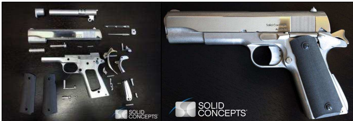
Figure 1: Fully functional 3D printed 1911 by Solid Concepts (Stratasys).
