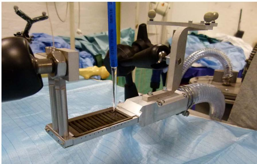
**Figure 4.** Prototypic jet absorber for the clinic AWIJ application
