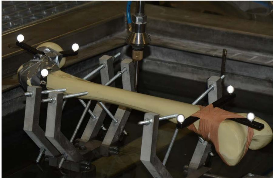
**Figure 5.** Mounted reflecting reference marks on an artificial bone
