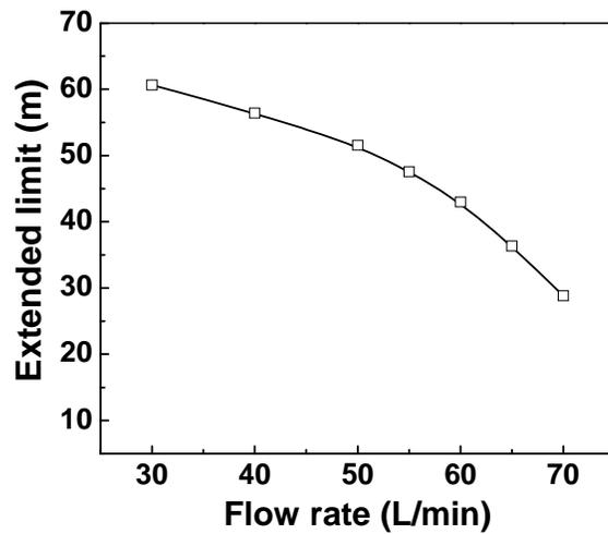
Figure 6. Relationship between flow rate and extended limit of horizontal well
