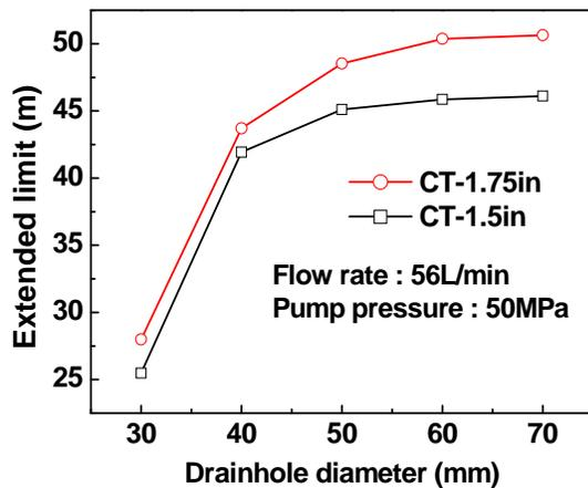
**Figure 11.** The effect of well diameter
