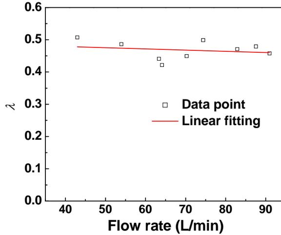
**Figure 5.** Relationship between flow rate and coefficient- $\lambda$
