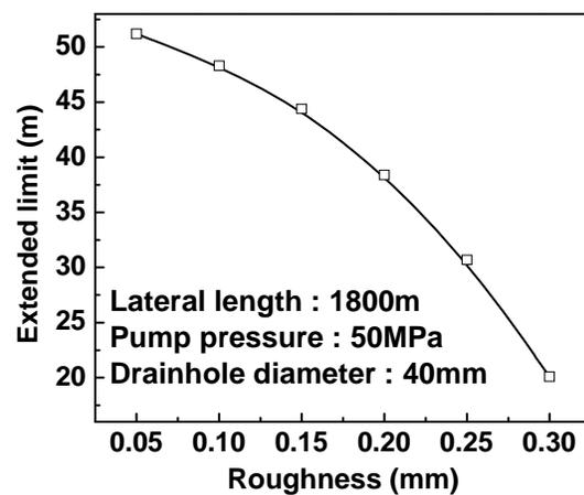
**Figure 8.** Effect of well roughness
