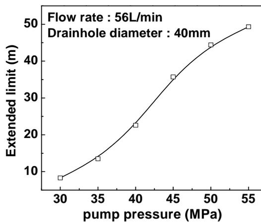
**Figure 7.** Effect of pump pressure
