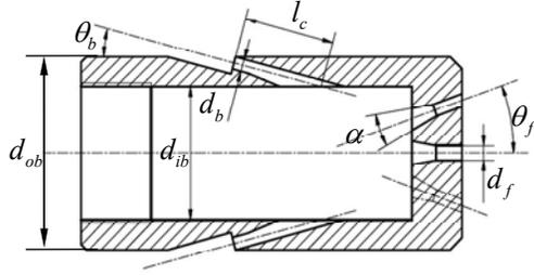
**Figure 2.** Structure diagram of jet nozzle
