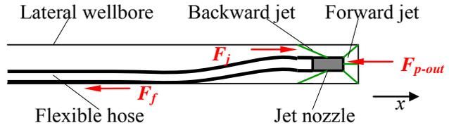
**Figure 3.** Force analysis of drilling system
