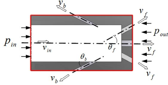
**Figure 4.** Fluid flowing state within jet nozzle
