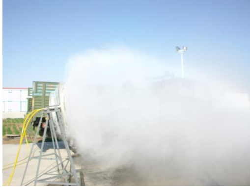
Figure 10 in the two-level wind weather conditions mist shielding effect
