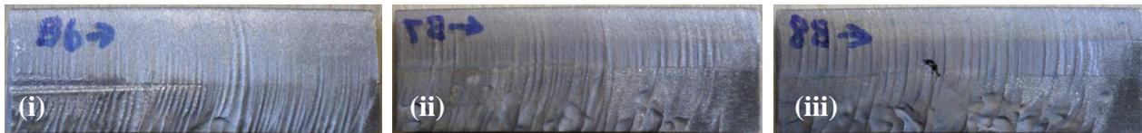
**Figure 14** Traverse speed ( $V_t$ ) with  $m_a = 490$  g/min (i) 200 mm/min (ii) 220 mm/min (TC) (iii) 240 mm/min (non-TC)
