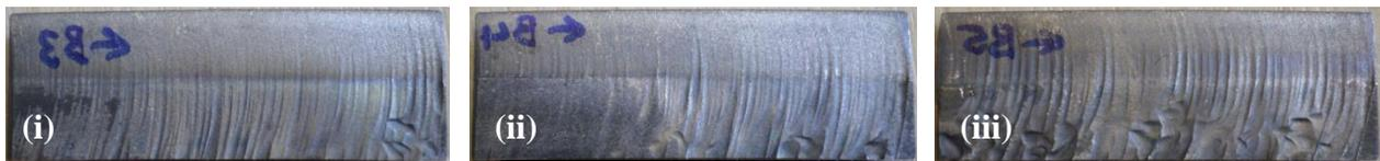
**Figure 13** Traverse speed ( $V_t$ ) with  $m_a = 300$  g/min (i) 160 mm/min (ii) 180 mm/min (TC) (iii) 200 mm/min (non-TC)
