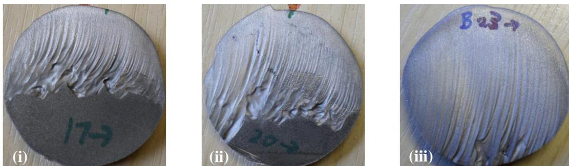
**Figure 8** Cylindrical cut face after varying  $V_t$  (i) 200 mm/min (ii) 140 mm/min (iii) 80 mm/min
