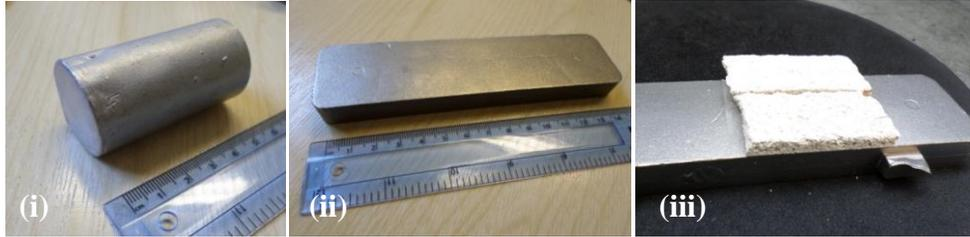
**Figure 1** Test specimens prior to cutting (i) 30 mm diameter cylinder (ii) 13 mm thick plate (iii) refractory coated specimen
