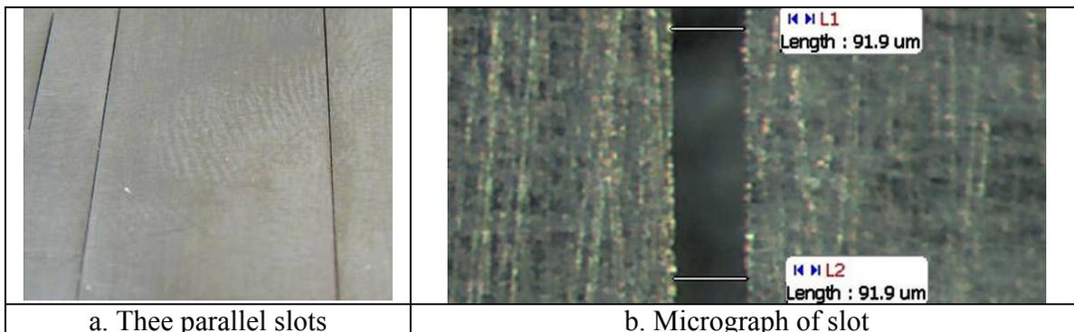
Figure 4. AWJ-machined narrow slots using a novel auxiliary device (patent pending)
