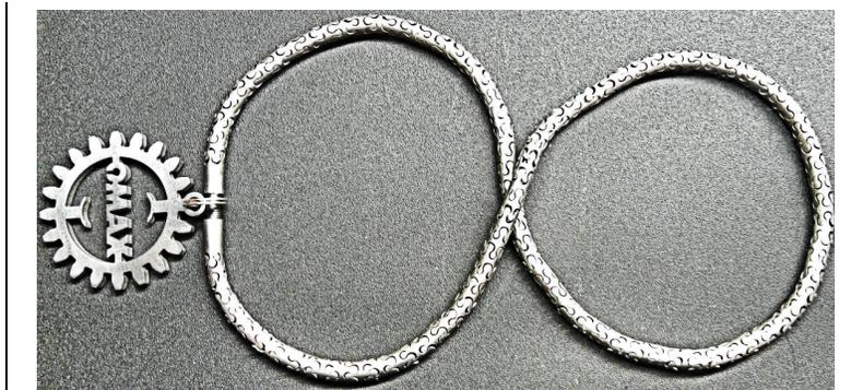
**Figure 13. AWJ-machined interlocking link made from a solid titanium tube (0.64 mm OD)**
