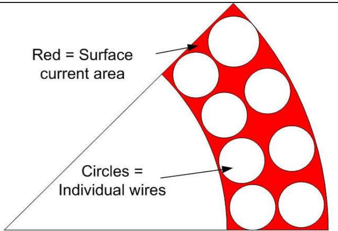
**Figure 6. Schematic of multi-round-turn conductor**
