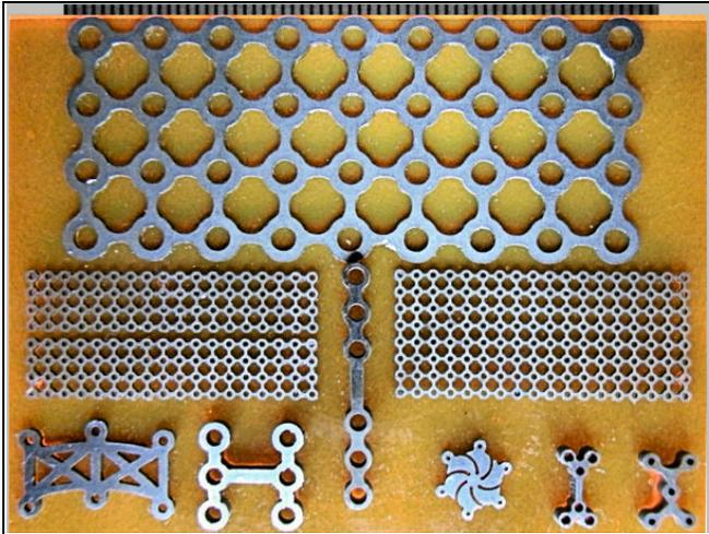
Figure 10. AWJ-machined orthopedic components – scale in mm
