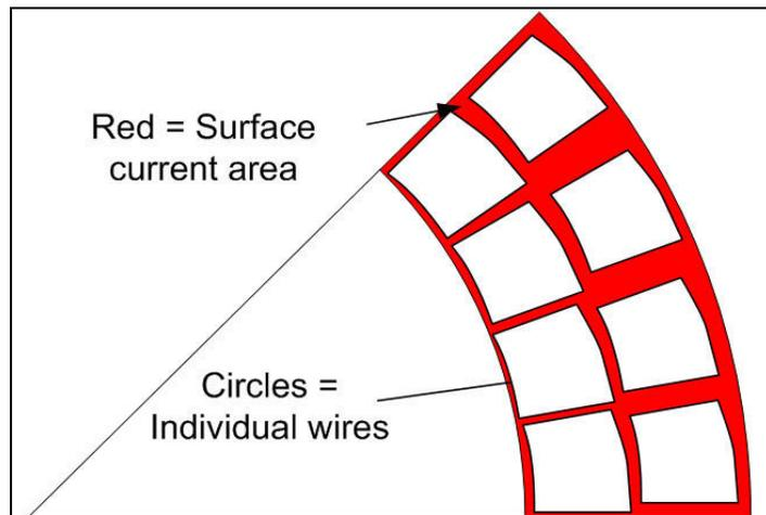
**Figure 7. Schematic of multi-square-turn conductor**
