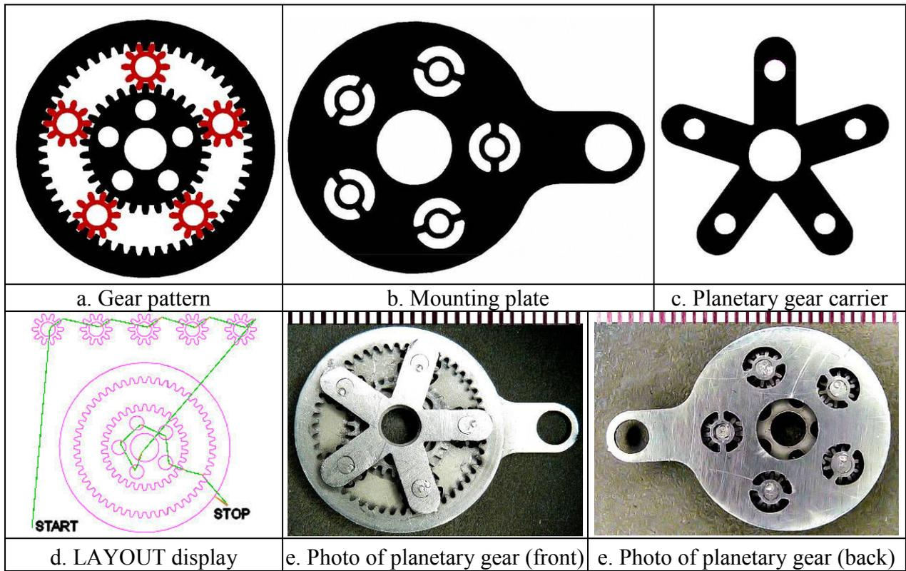
Figure 12. AWJ-machined stainless steel planetary gear set – scale in mm
