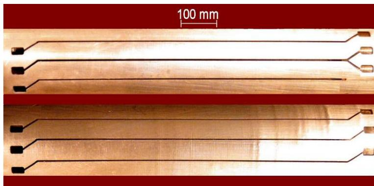
**Figure 9. Sections of AWJ-slotted copper tubes (slot patterns provided by PERG at MIT (<http://pergatory.mit.edu/>))**
