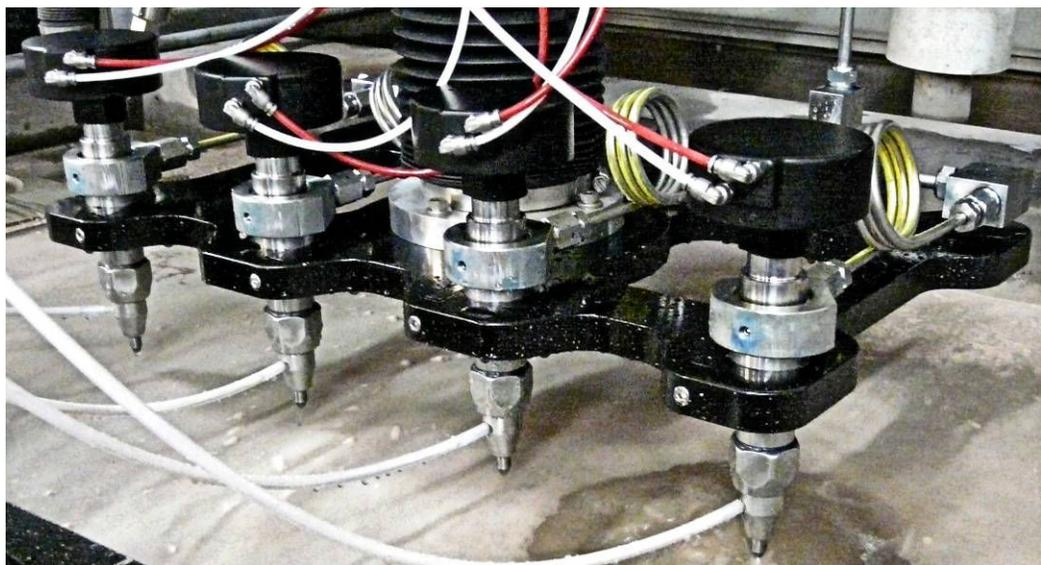
**Figure 14. Multi-nozzle platform accommodating four beta 5-10 nozzles operating in tandem**
