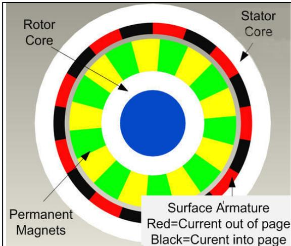
**Figure 5. Typical configuration for a permanent magnet motor/generator**
