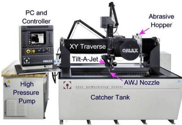
Figure 1. Model 2652 JetMachining Center
