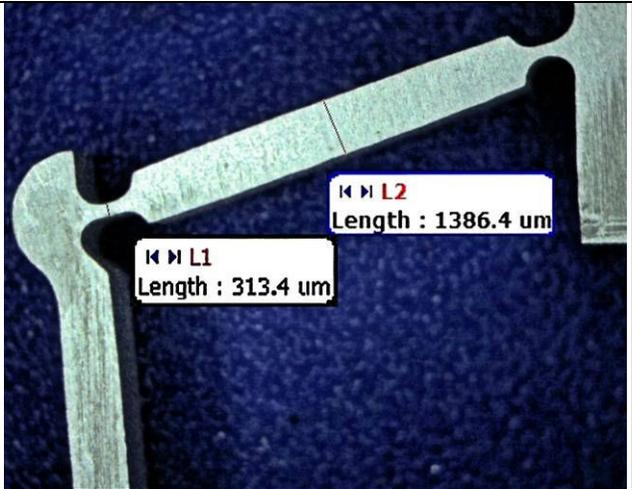
Figure 11. Mean features of a small flexure for a medical device (PERG at MIT)
