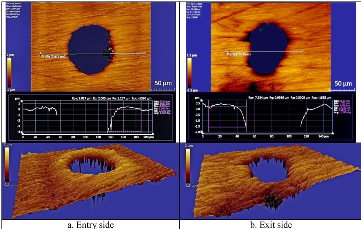
Figure 3. Micrographs of the hole pierced on 316 stainless steel shim - courtesy of Zygo Corp and Microproducts Breakthrough Institute
