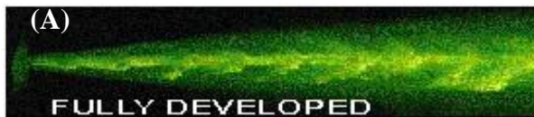
Figure 3. Typical appearance of HFPWJ. (A) Issuing from a single-orifice nozzle, (B) Issuing from a dual-orifice nozzle.
