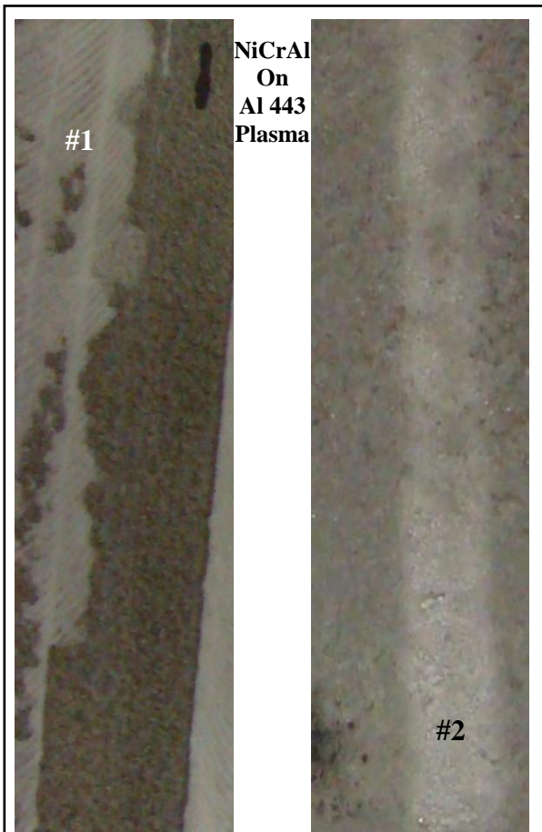
Figure 11. Stripping with UHPCWJ (#1) and HFPWJ (#2).
