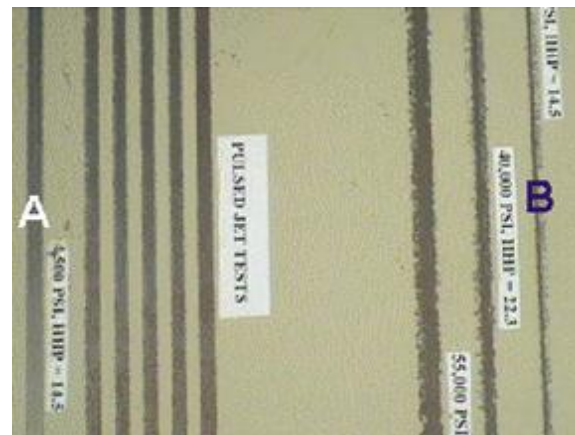
Figure 5. Baked enamel stripped from a steel plate. (A) HFPWJ @ 31-MPa (10.8-kW), (B) UHPCWJ @ 207-MPa (10.8-kW).
