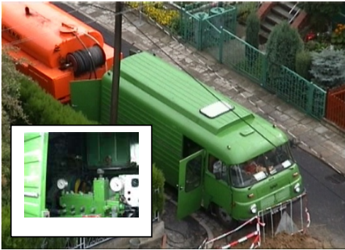
Fig. 11. General view of two mobile test stands based on a hydro monitor with a high-pressure pump
