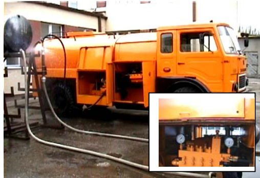
Fig. 11. General view of two mobile test stands based on a hydro monitor with a high-pressure pump
