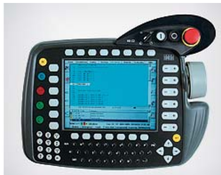
Figure 4: Typical hand held teach pendant hardware for Point-to-Point teaching
