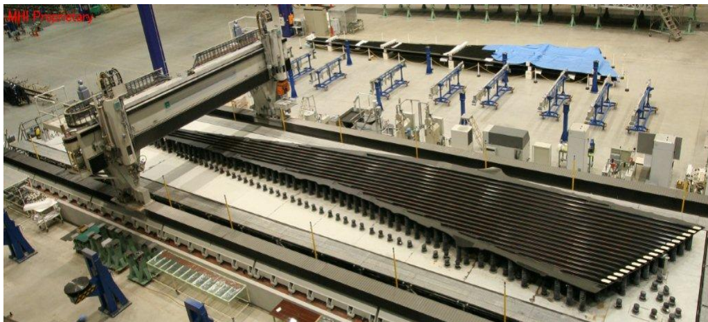
Figure 2: Large Gantry for Boeing 787 Wing Trimming
