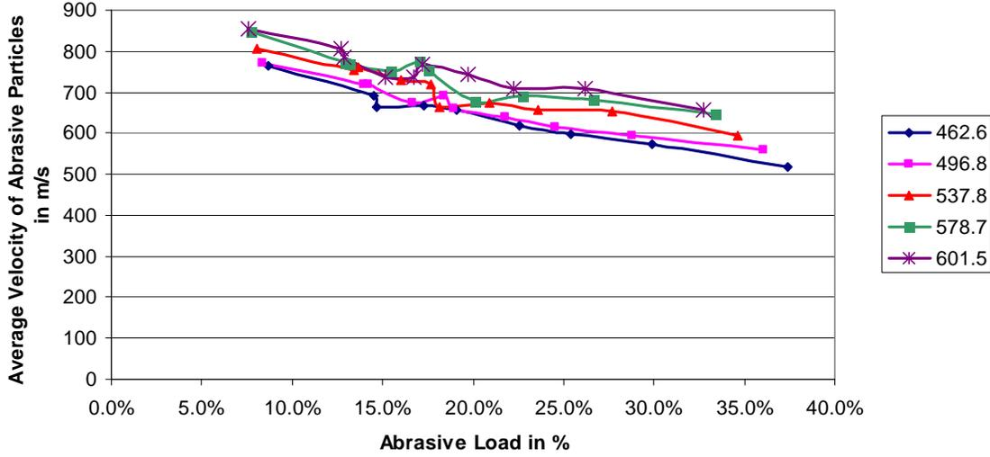
Figure 1. Particle Velocity at different water pressures over Abrasive Load ( $d_o=250\mu\text{m}$ ,  $d_r=760\mu\text{m}$ )
