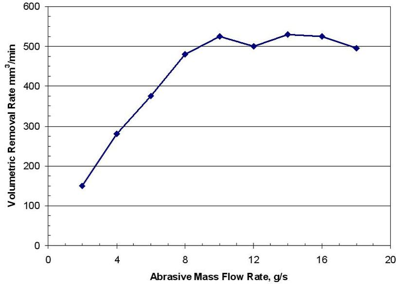
Figure 4: Volumetric material removal rates as a function of abrasive mass flow rates on steel [13] ( $d_o=250\mu\text{m}$ ,  $d_f=900\mu\text{m}$ ,  $P=300\text{ MPa}$ ).
