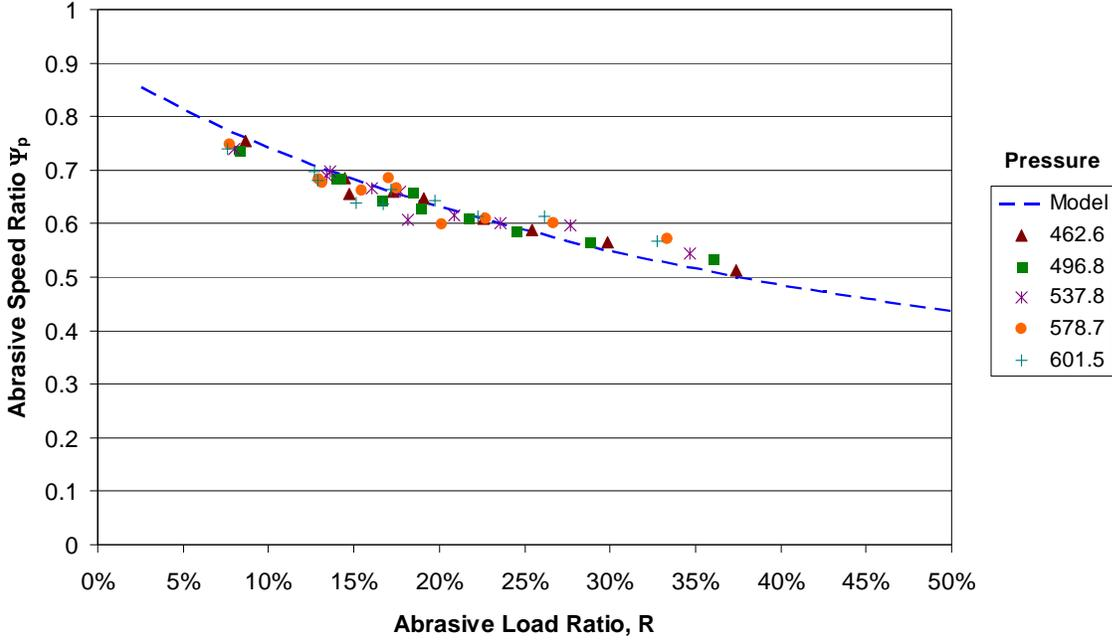
Figure 2. Experimentally determined Abrasive Speed Ratio at different Pressures ( $d_o=250\mu\text{m}$ ,  $d_f=760\mu\text{m}$ )
