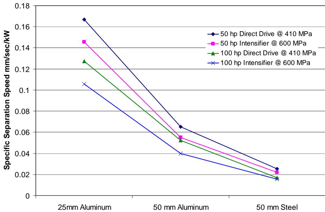
50 hp Direct Drive:  $d_o = 381 \mu\text{m}$ ,  $\dot{m}_a = 6.1 \text{ g/s}$       100 hp Direct Drive:  $d_o = 559 \mu\text{m}$ ,  $\dot{m}_a = 10.6 \text{ g/s}$
