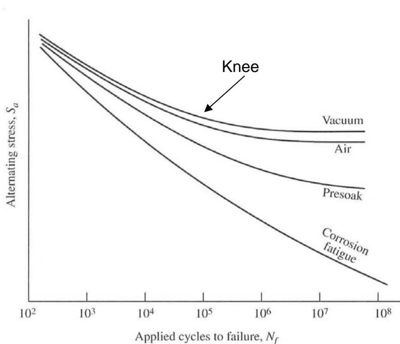
Figure 7: Typical fatigue behavior in different environments [16].
