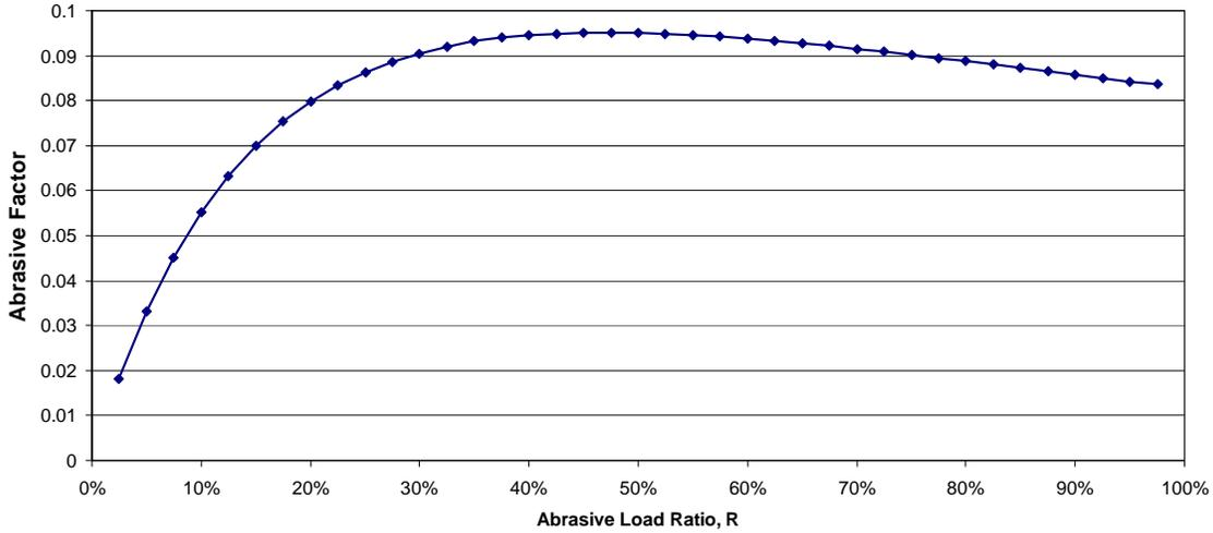
**Figure 3. Abrasive Factor as a function of Abrasive Load Ratio with  $R_{MAX}=47\%$**
