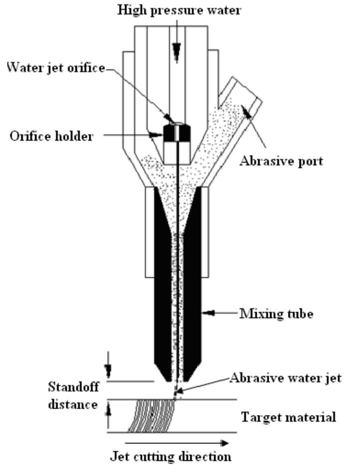
**Figure 1.** Schematic diagram of Abrasive water jet machining.
