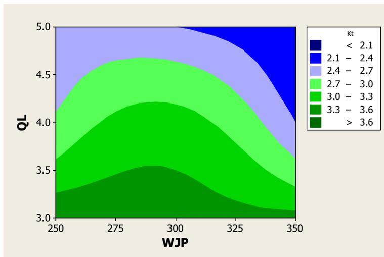
**Figure 8.** 3-D Contour plots showing the interaction effect of WJP and QL on  $R_a$  and  $K_t$ .
