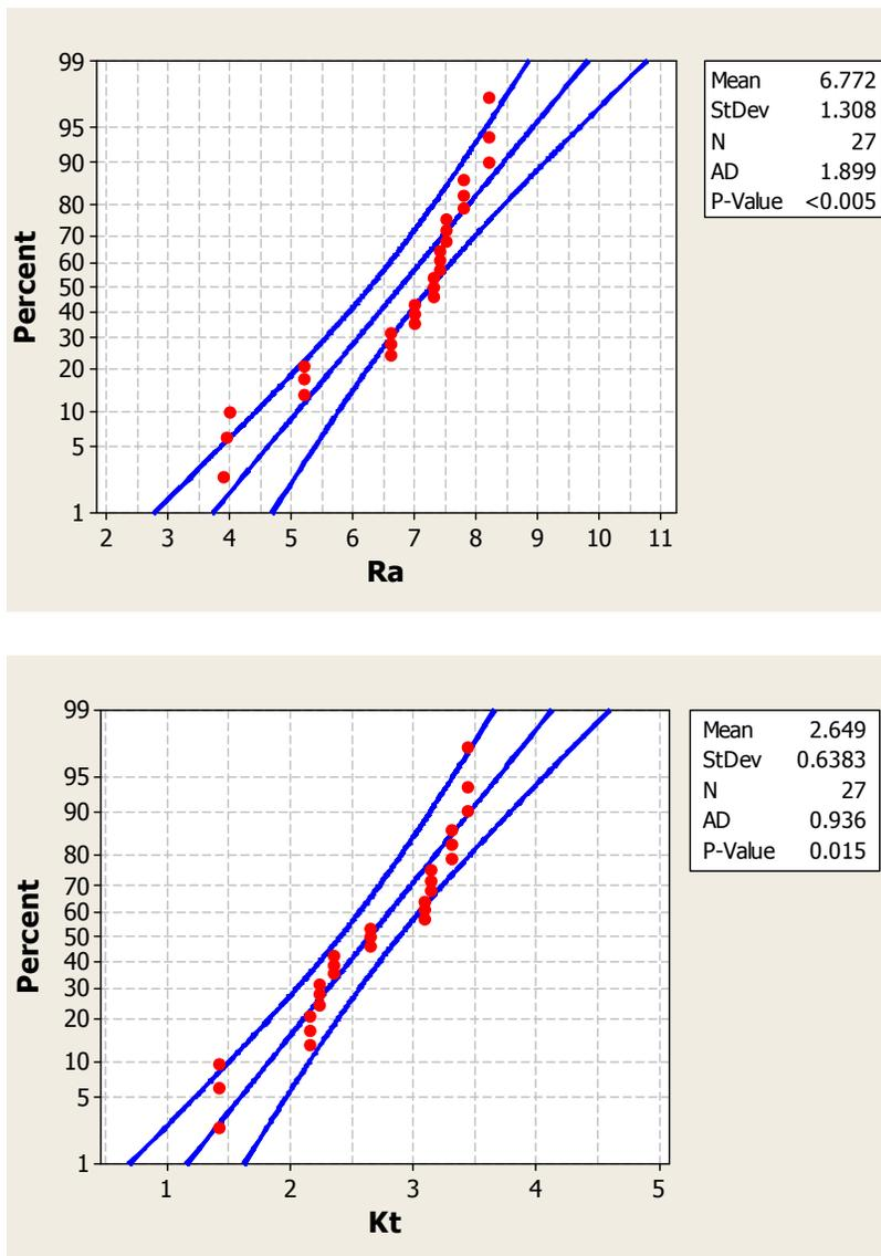
Figure 7. Normal probability plot of  $R_a$  and  $K_t$  (for Kevlar/epoxy composite).
