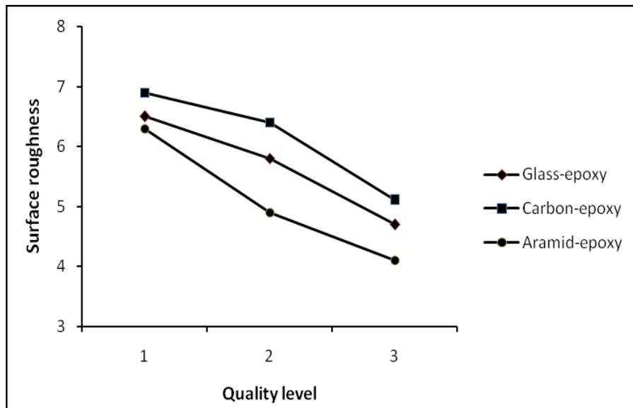
**Figure 2.** Effect of different quality levels (3, 4 and 5) on Surface roughness for three composite.
