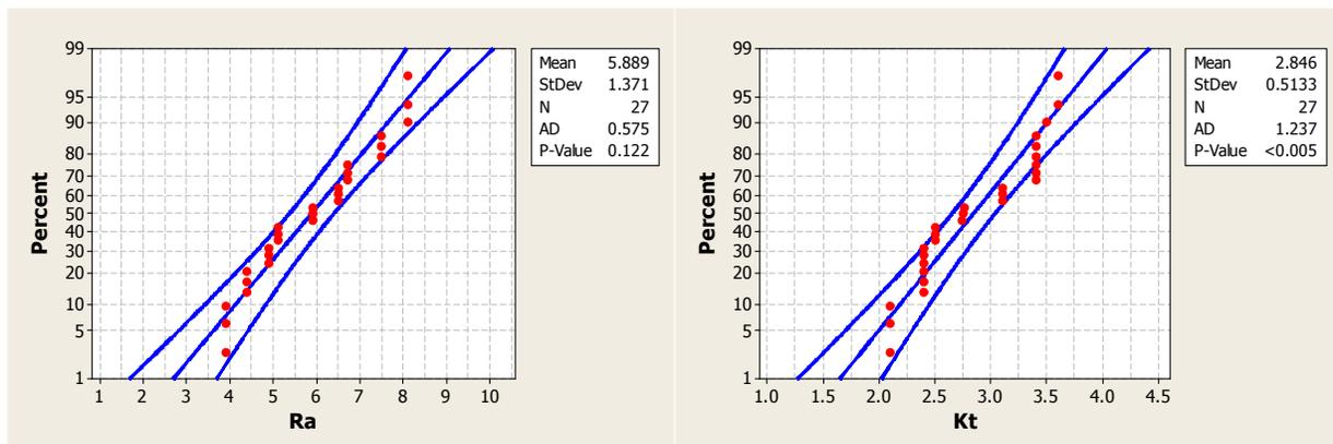
**Figure 5.** Normal probability plot of  $R_a$  and  $K_t$  (for glass/epoxy composite).
