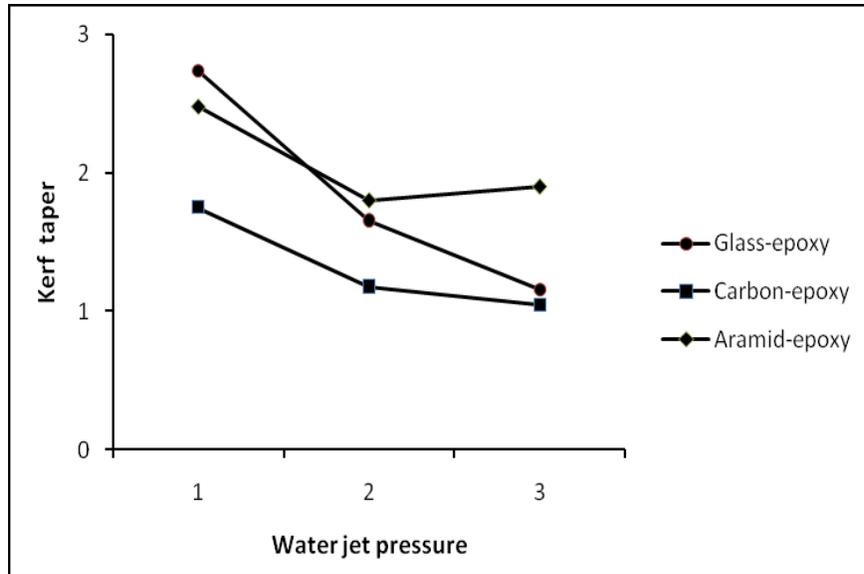
**Figure 3.** Effect of waterjet pressure (250, 325 and 400 MPa) on Kerf taper for three composite.
