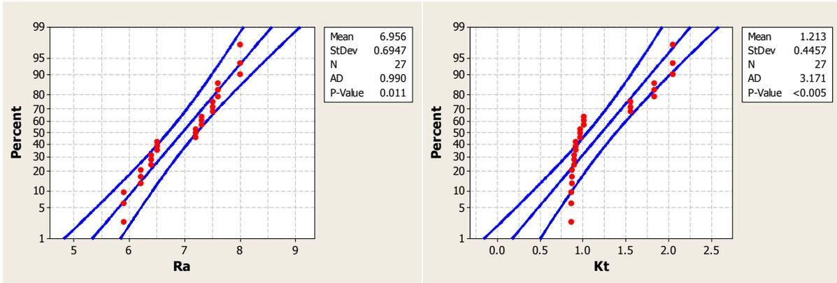
Figure 6. Normal probability plot of  $R_a$  and  $K_t$  (for carbon/epoxy composite).
