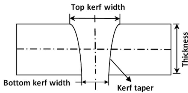
**Figure 4.** Schematic diagram of AWJ cut kerf geometry.
