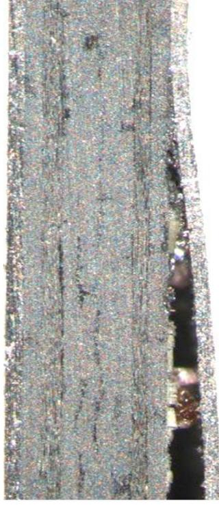
Abrasive Embedment and Delamination at the Jet Exit
