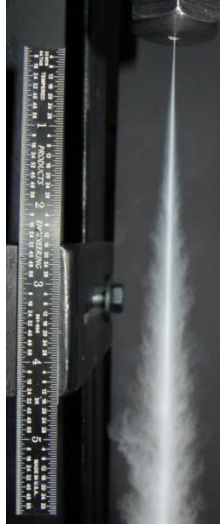
Figure 1. Image depicting jet structure for a WJ operating at 600 MPa. ( Scale in inches )
