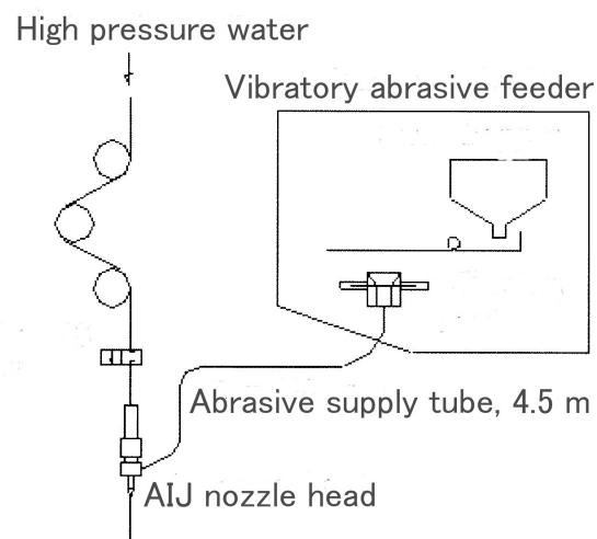
**Figure 1:** Schematic diagram of the water jet machining system
