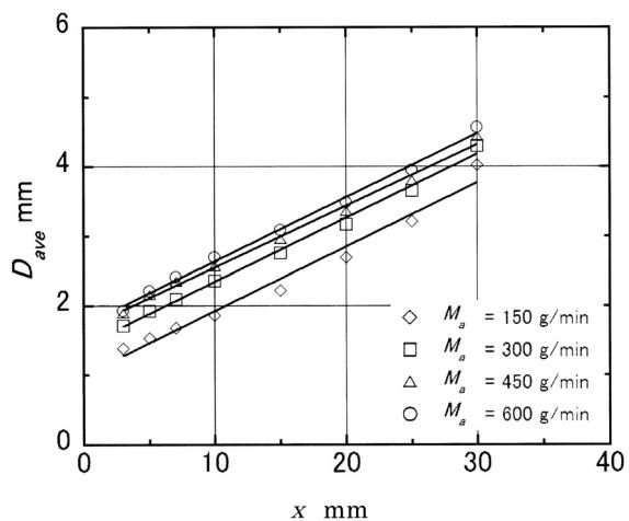
**Figure 3:** Variation of time averaged jet diameter with standoff distance ( $p_i = 300$  MPa)
