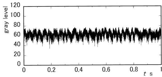
**Figure 7:** Time variation of the jet gray level at 7 mm downstream of the focusing nozzle exit ( $p_i = 300 \text{ MPa}$  and  $M_a = 300 \text{ g/min}$ )
