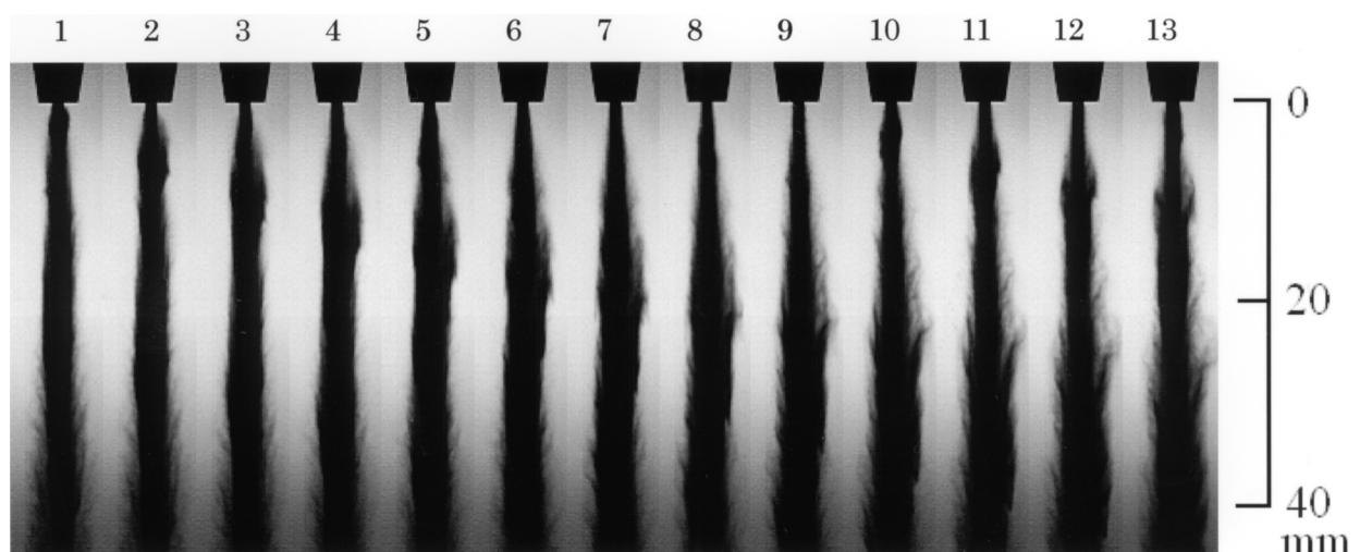
**Figure 2:** Time series of photographs of AIJ ( $p_i = 300$  MPa and  $M_a = 600$  g/min)
