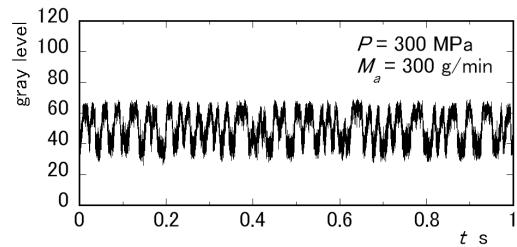
**Figure 9:** Time variation of the gray level in the abrasive supply tube at 2 mm upstream of the abrasive port ( $p_i = 300 \text{ MPa}$  and  $M_a = 300 \text{ g/min}$ )
