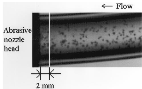
**Figure 5:** Flow in the abrasive supply tube ( $p_i = 300$  MPa and  $M_a = 300$  g/min)
