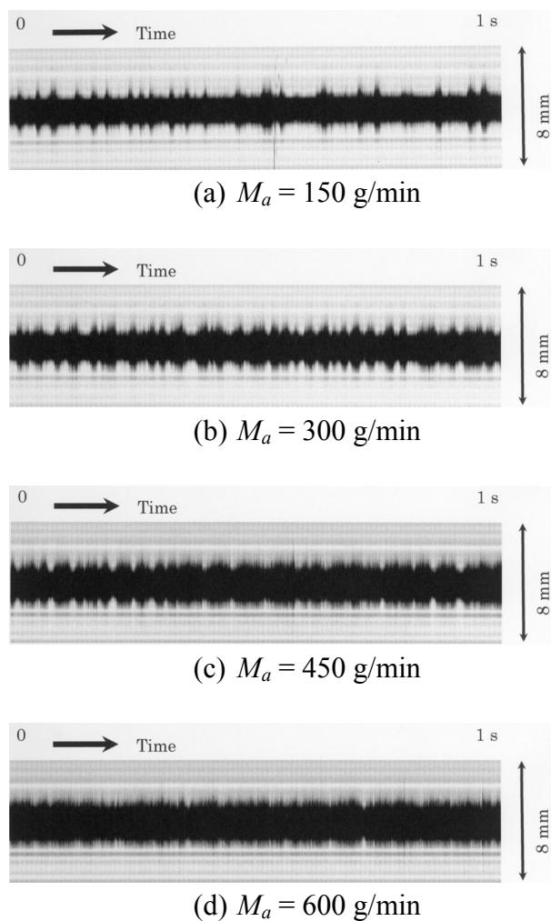
**Figure 4:** Time series image of the jet boundary at  $x = 7$  mm and  $p_i = 300$  MPa
