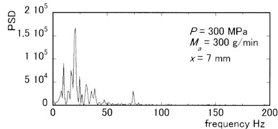
**Figure 8:** Power spectrum of the jet gray level at 7 mm downstream of the focusing nozzle exit ( $p_i = 300 \text{ MPa}$  and  $M_a = 300 \text{ g/min}$ )
