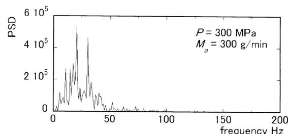
**Figure 10:** Power spectrum of the gray level in the abrasive supply tube at 2 mm upstream of the abrasive port ( $p_i = 300 \text{ MPa}$  and  $M_a = 300 \text{ g/min}$ )
