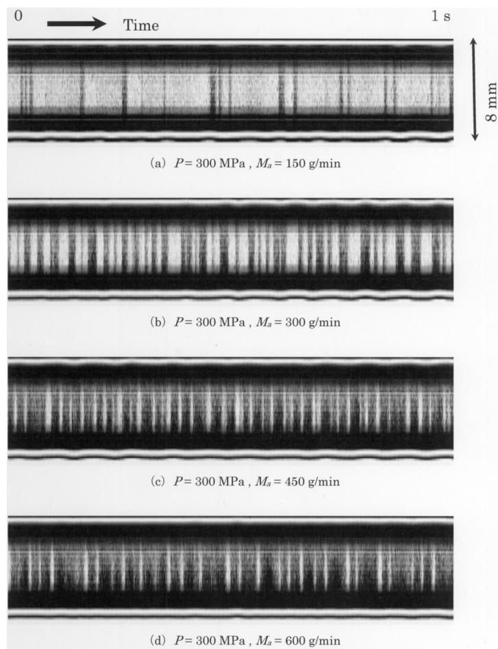
**Figure 6:** Time series image of the flow in the abrasive supply tube at 2 mm upstream of the abrasive port ( $p_i = 300$  MPa)
