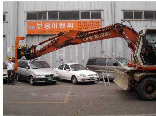
Figures 2.2 & 2.3 Diajet Mixer with Pump used in Field Test with Excavator
