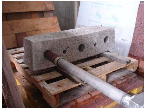
Figures 3-2 & 3-3 Portable Disking Nozzle Head and A View Placed inside a Cored Hole
