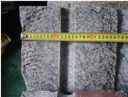
Figure 4-10 & 4-11 Notching Test & Notching Direction Marking
