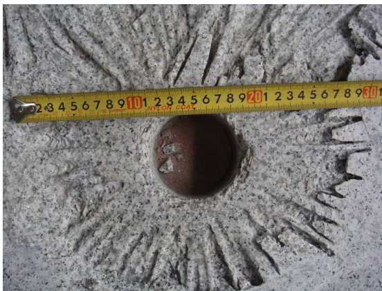
Figure 3-6, 3-7 Disked Rock : Individual Disk Cross Section & Split Apart Rock Block
