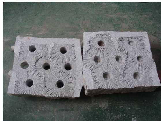
Figure 3-6, 3-7 Disked Rock : Individual Disk Cross Section & Split Apart Rock Block
