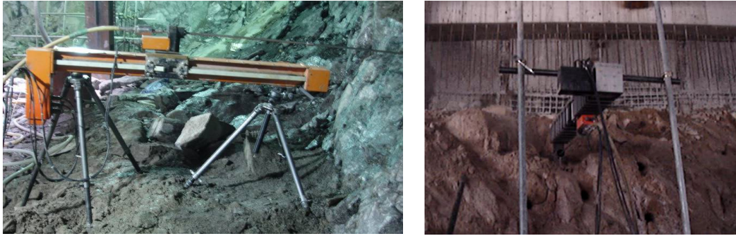
Figures 2.4 & 2.5 System mount on tripods and bars-pipes
