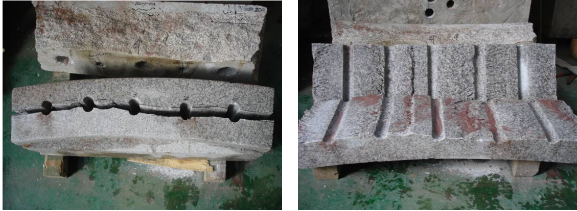
Figures 4-12 & 4-13 Notch Cuts Connected & Split View
