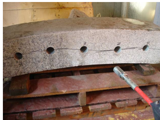
Figure 4-10 & 4-11 Notching Test & Notching Direction Marking
