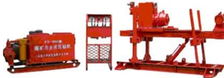
Figure 7. ZY-1250 fully hydraulic drill for coal mine
