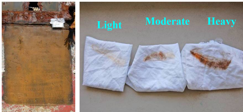
Figure 12 Moderate Rust.- little to no black rust under the brown rust Comparison of Light, Moderate, and Heavy Flash Rust.
