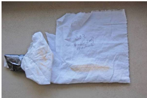
Figure 13 Moderate Flash Rust, Swatch and Brush Wipes
