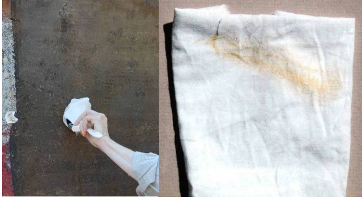
Figure 11 Brush Test. A little color is transferred.
