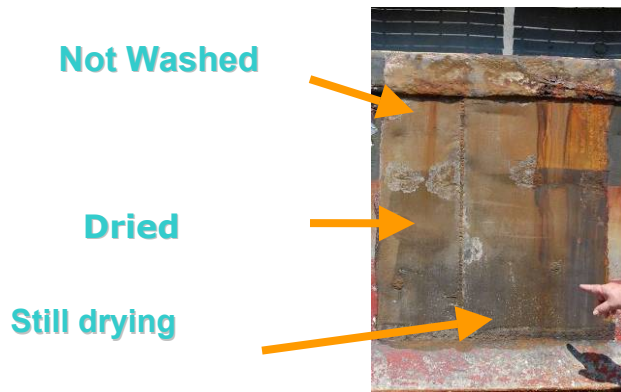
Figure 14 Heavy Flash Rust Comparison Swatch, Brush, wipe
