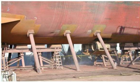
Figure 1 Flash Rust and Rust Back
