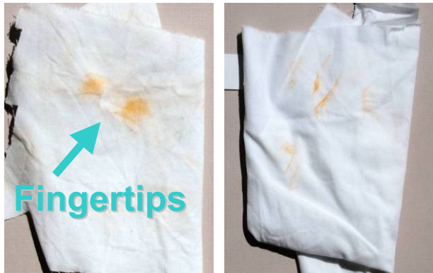
Figure 6 Light Flash Rust. Fingertips met the surfaces. Small color transference.
