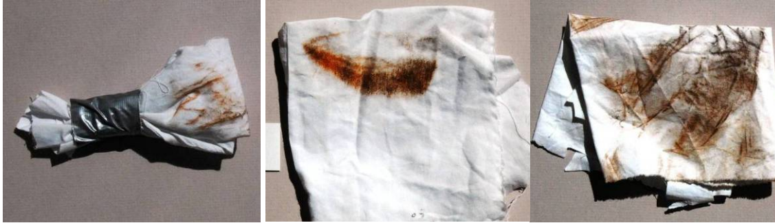
Figure 14 Heavy Flash Rust Comparison Swatch, Brush, wipe
