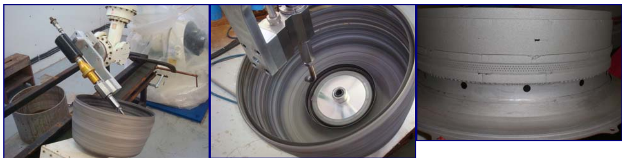
Figure. 13. Stripping of a variety of aircraft parts with the specially designed FPWJ nozzles. The third photograph shows a close-up view of the part from which TBC coating was removed.
