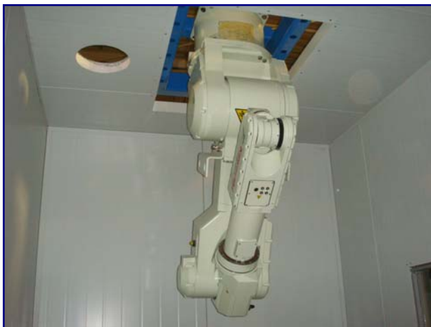
Figure 5. A close-up view of the Kawasaki robot mounted on the ceiling of the booth
