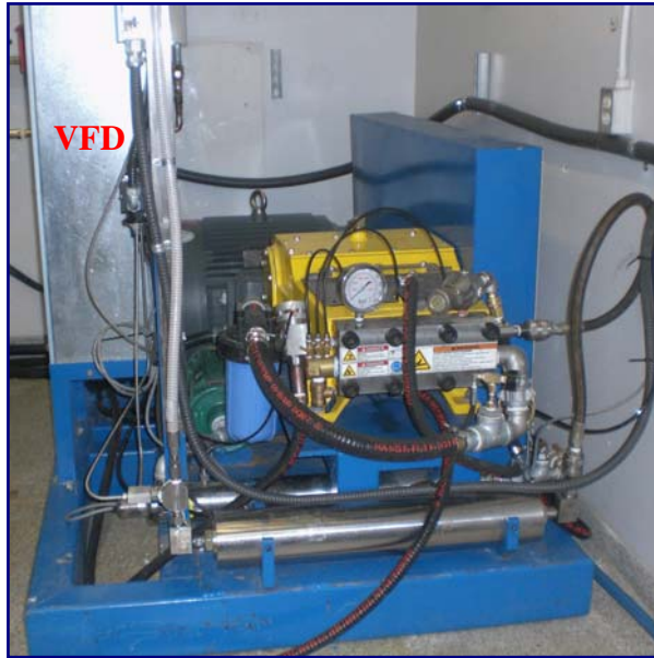
Figure 7. A general view of the Jetstream pump controlled by the VFD.
