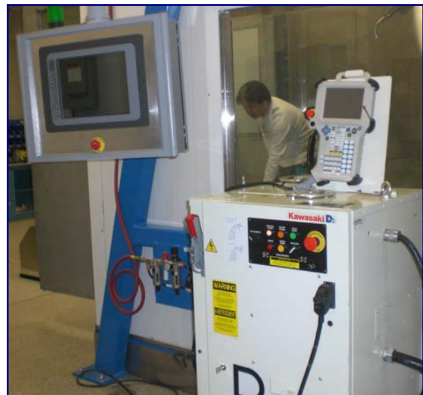
Figure 10. General view of the HMI and robot control box located near the window of the booth.
