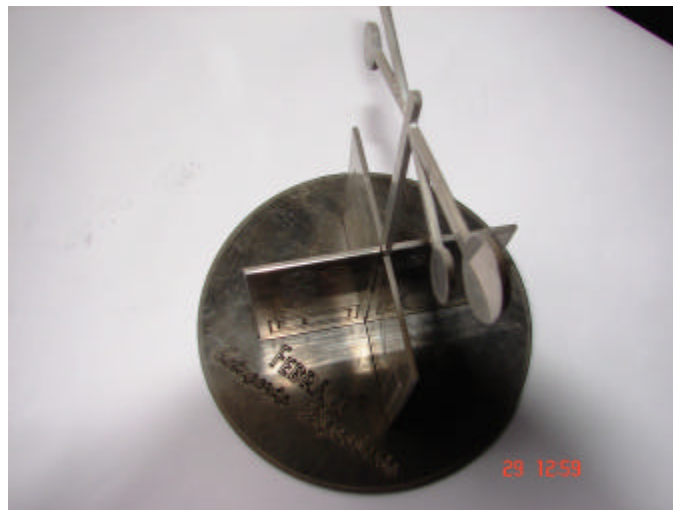
Figure 11. FEBRACE 4 th photography etch and cut by sbrasive waterjet.
