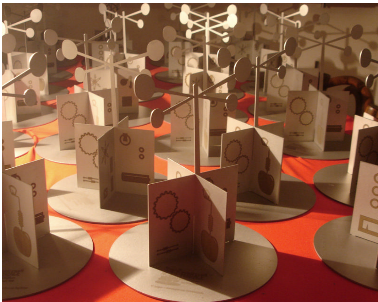
Figure 16. Stainless steel trophy after laser milling.
