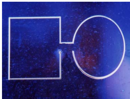
Figure 8: Good top surface quality cut in 'flashed' glass during the curves and arcs cutting trial.
