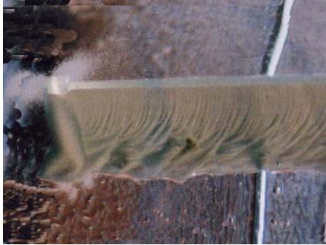
Figure 5: A rotating pierce with some residual blasting and uneven taper to the cutting. The pierce itself is good but the cut is poor.
