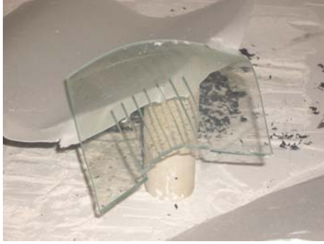
Figure17: ‘Informed play’ using waterjet cuts into glass. Placing glass into the kiln and to see how the glass can be manipulated into various different shapes. Waterjet lines into the glass could react differently to a waterjet cut shape.
