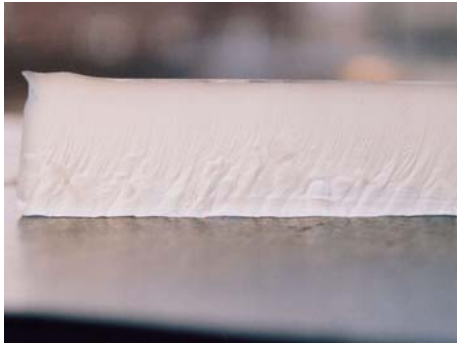
Figure 3: An example of a poor quality cut visible, taper uneven of cut, striations. The taper of the jet path can be seen with glass virtually breaking away from its self. The kerf is noticeably visible. The jet appears to have struggled to get through the glass.
