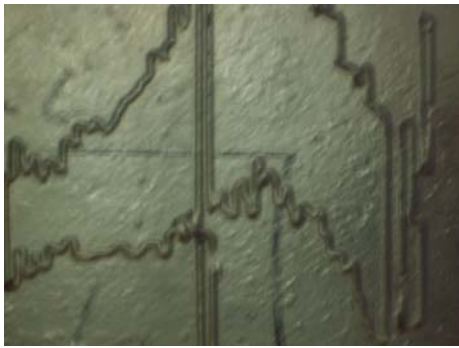
Figure 23: Detail of experimental milling into glass, work for Kathryn Hodgkinson 2006
