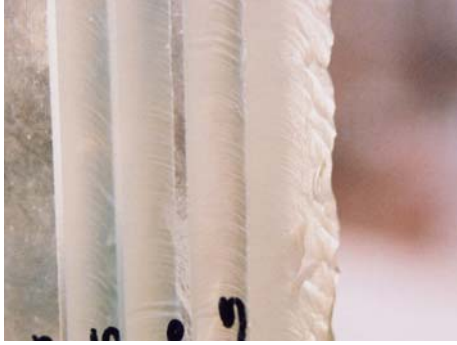
Figure 1: A series of poor quality cuts. Tapering, striations towards the underside of the glass.
