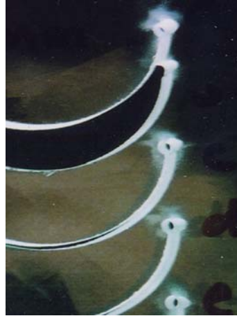
Figure 6: Several pierced holes on soda-lime (float) glass with residual blasting on the surface of the glass around the pierce hole.
