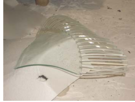
Figure 18: ‘Informed play’ using waterjet cut shapes. Placing into the kiln to see how the waterjet is affected by heat and being placed at irregular angles.
