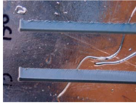
Figure 10: An example of a good quality pierce in 30mm thick cast glass. The lower cut in the picture shows the pierce looking through the glass surface. The pierce is straight, with no residual blasting or flaving around the entry point. The abraded surface is smooth and without distortion. In the top pierce there is some noticeable residual basting on the surface of the glass.
