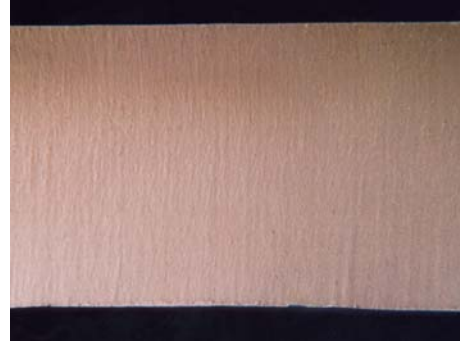
Figure 2: A good quality cut, no striations, taper or roughness.
