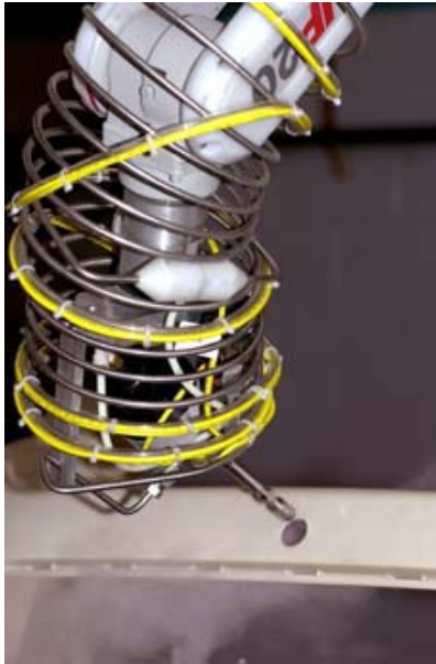
Figure 3. Compound angle circle cutting
