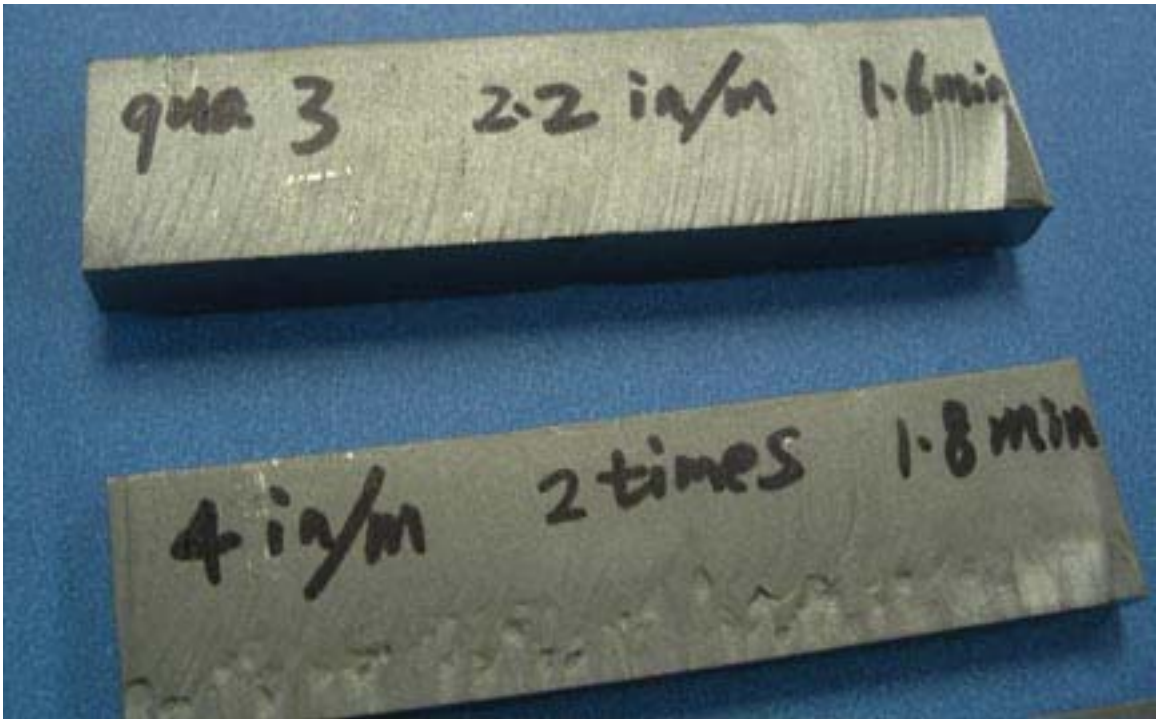
Figure 3. Cut edge quality at 5.5 and 10 cm/min speed.
