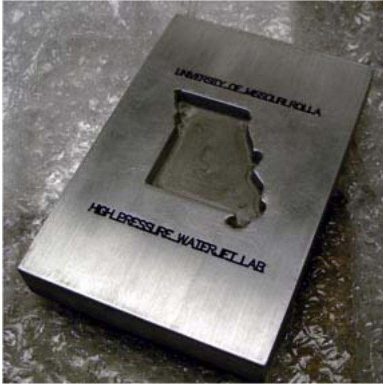
Figure 7. Milled map of Missouri showing the flat bottom of the milled pocket.
