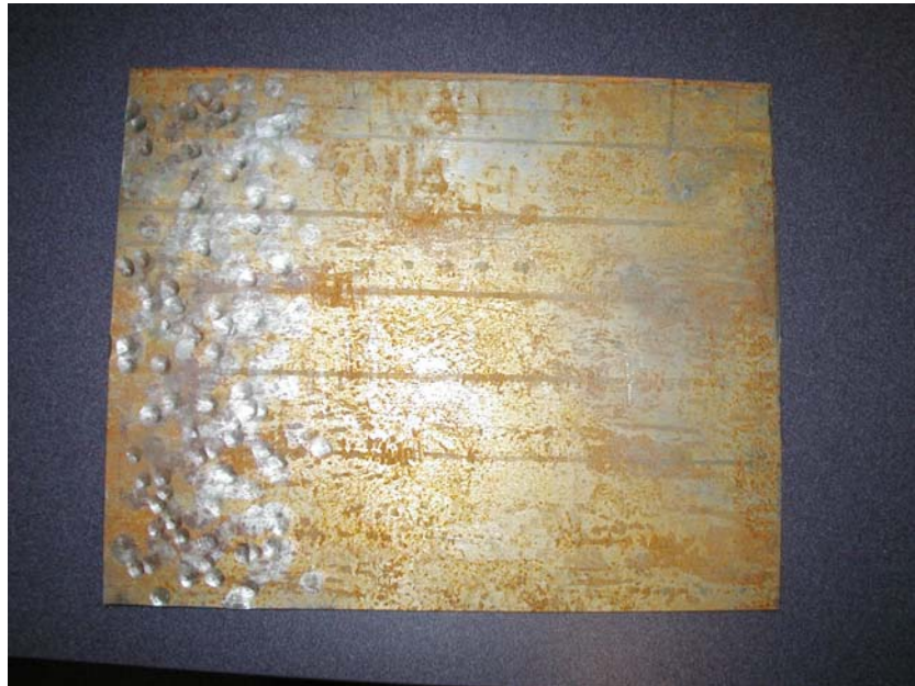
Figure 1. Steel plate was hammered to create residual stresses.
