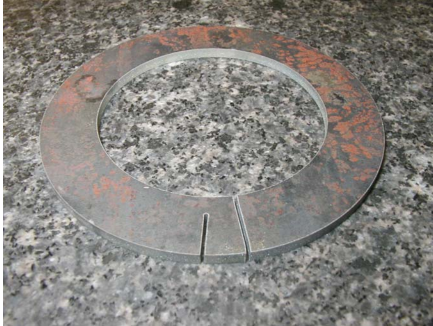
Figure 9. Split ring cut on stress relieved material.
