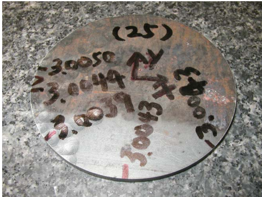
Figure 5. Disc cut on the hammered plate with stress relief.
