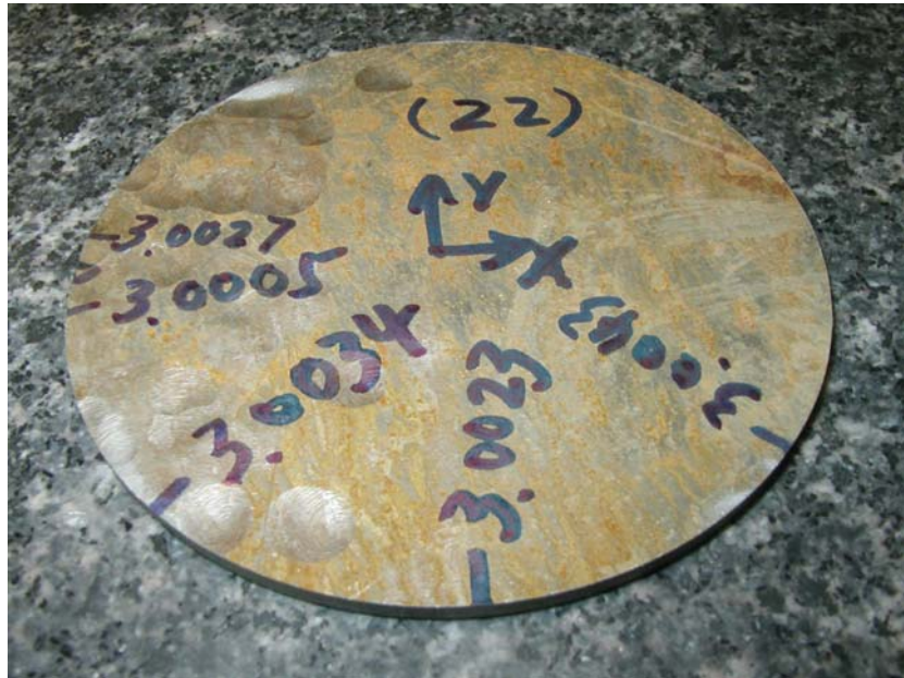
Figure 2. Disc cut on the hammered portion of the steel plate.
