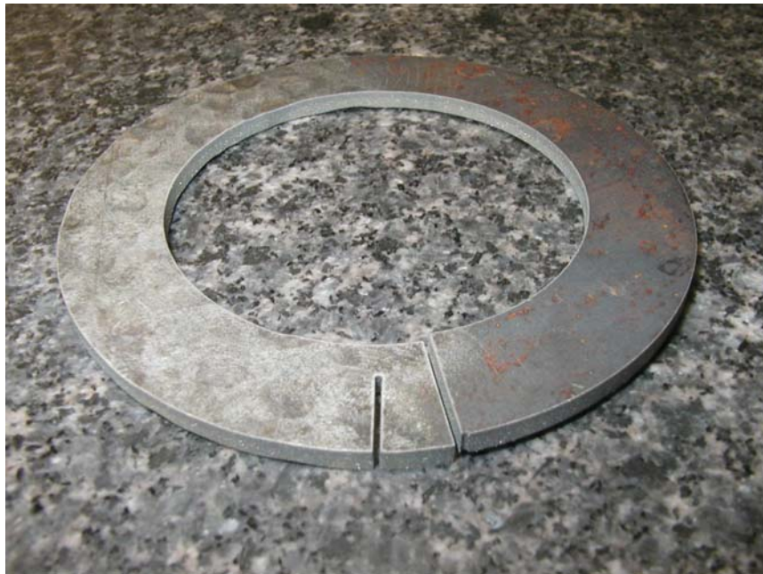
Figure 10. Split ring cut on material having residual stresses.
