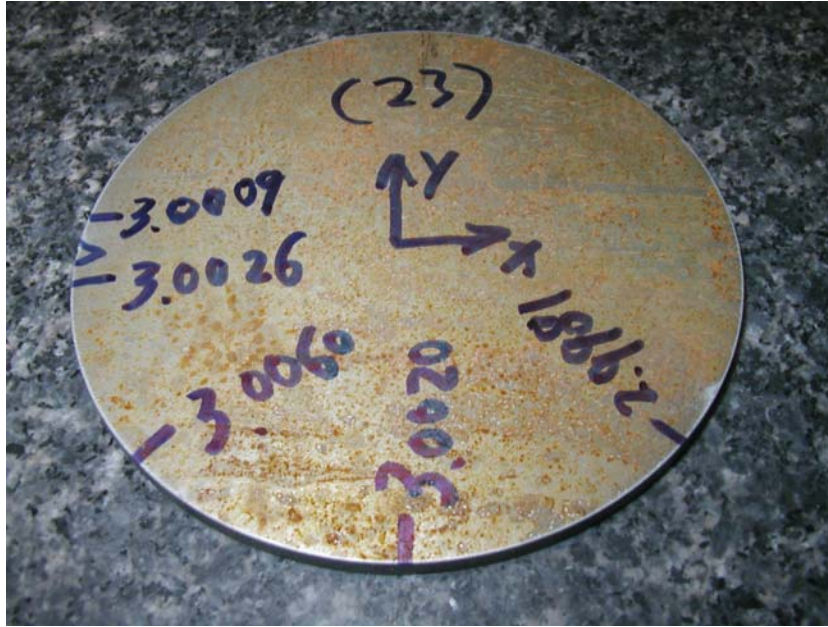
Figure 3b. Disc cut through the edge on the un-hammered portion of the steel plate.
