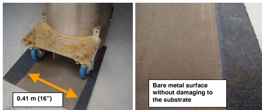
Fig. 7. Photograph showing the TURN set up for removing the non-skid coating from a steel panel at 10 kpsi (69
