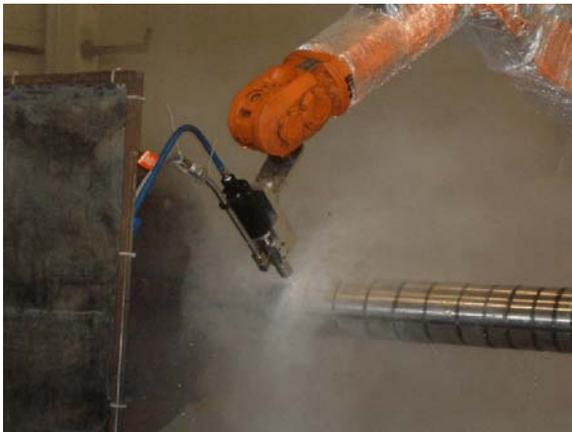
Fig. 3 Photograph showing the assembly of transducer (located in the black cylinder) and the nozzle mounted on a pedestal robot (courtesy of St. Louis Metallizing, USA).
