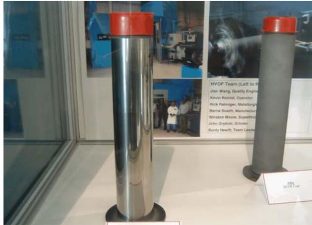
**Fig. 6 Highly polished (foreground) and HVOF (WC-Co-Cr) coated landing gear pins received from Messier-Dowty**
