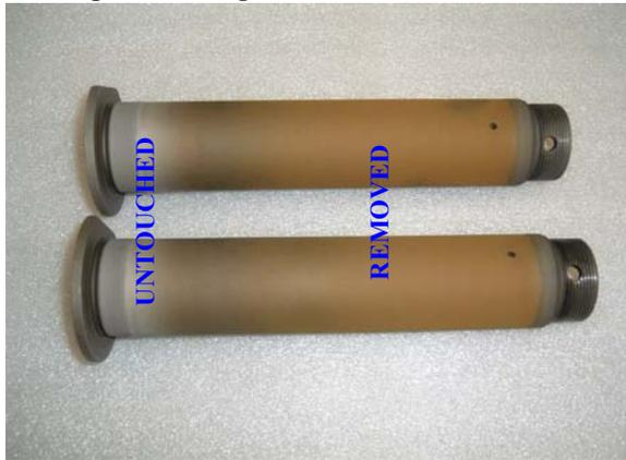
**Fig. 7 A general view of the landing gear pins from which the HVOF coatings were removed with the FPWJ. The untouched part was used for analysis by Messier-Dowty.**
