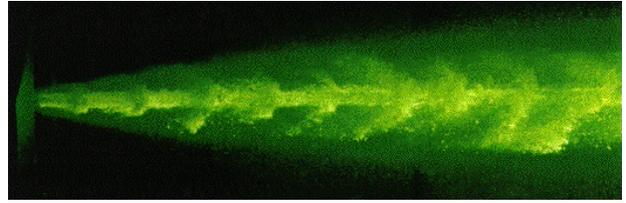
Fig. 1B Photograph of the well-defined and fully developed FPWJ taken with a pulsed Nd-Yag laser [3].
