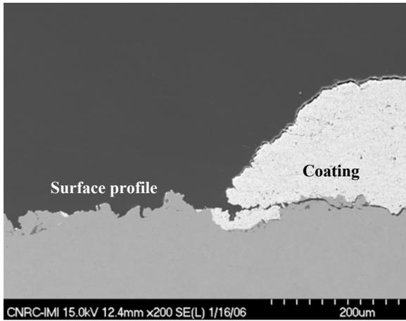
**Fig. 5 SEM view of the cross-section of the interface of coating and substrate showing the original grit-blasted profile.**
