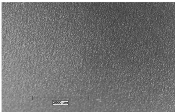
**Fig. 9 Typical surface finish of the pin observed with a stereoscope after stripping of the coating with FPWJ.**
