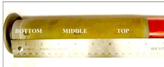
**Fig. 8 Location of probes for measuring the residual stresses along the pin after stripping with FPWJ using X-ray diffraction technique.**
