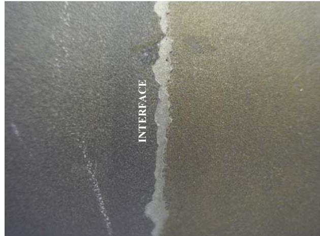
Fig. 4 Close up view of the coating (left) and substrate (right) showing the clean finish achieved with FPWJ stripping.
