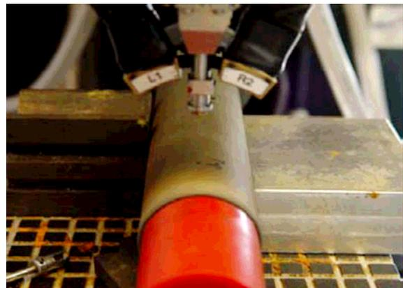
**Fig. 10 Set up of the pin in the X-ray machine for measuring residual stresses.**
