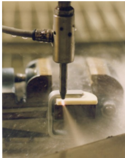
Figure 2. Cutting Translucent Aluminum Oxide (© Christian Ojmertz)
