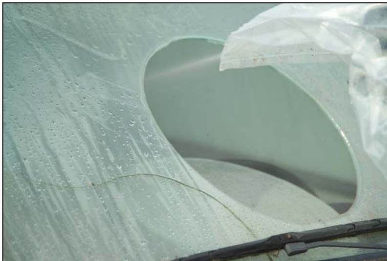
Figure 4. Successful cut of an access hole into a wind shield
