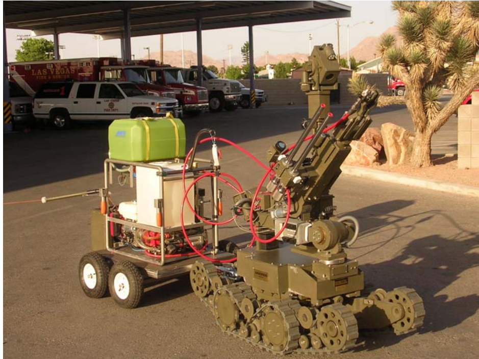
Figure 1. Remotec Mark-V robot with a mini MACE system on the trailer
