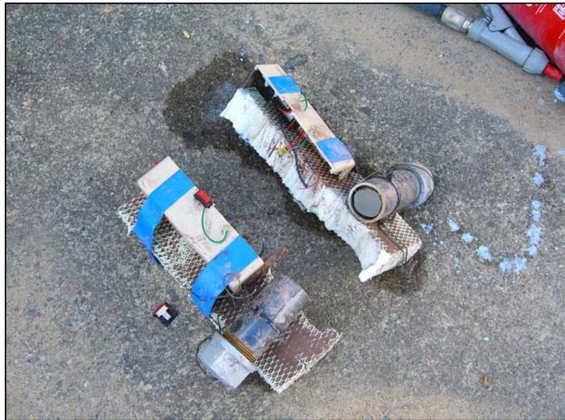
Figure 5. Successful cut through an IED with a pipe bomb
