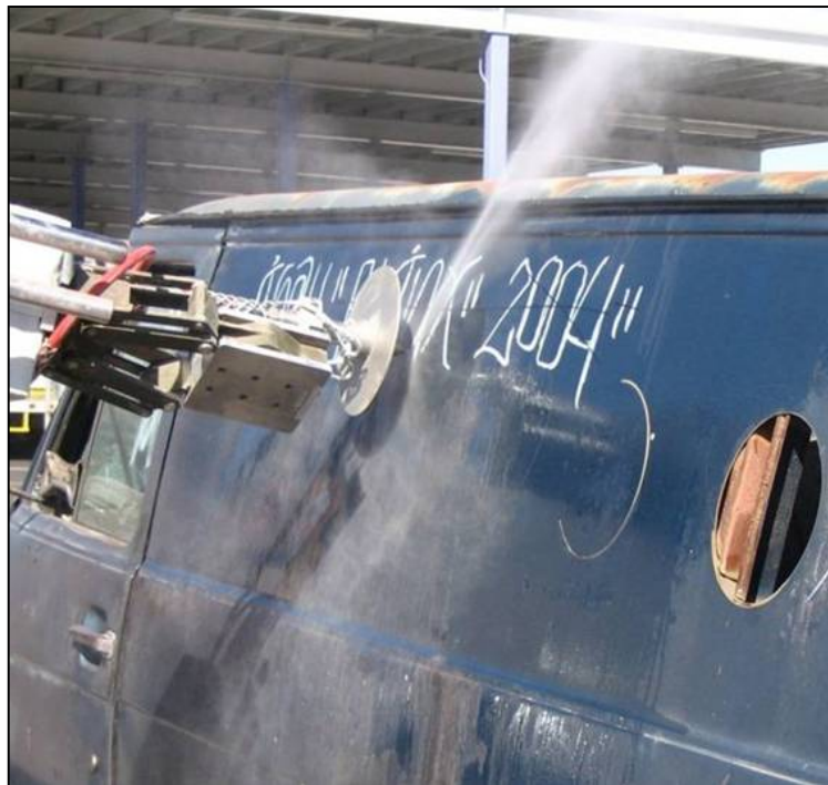
Figure 2. Cutting an access hole in the side of the van
