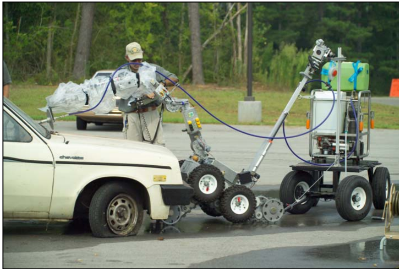
Figure 3. Test cut of a wind shield at HDS
