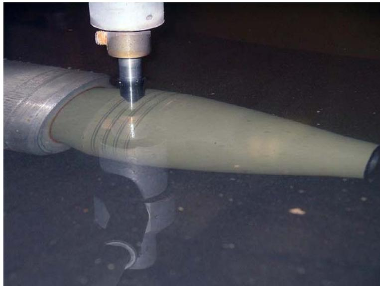
**Figure 4: Shell holding and rotation fixture used for experiments underwater.**
