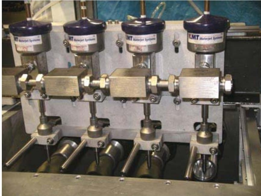
**Figure 3: Simplified current cutting arm.**
