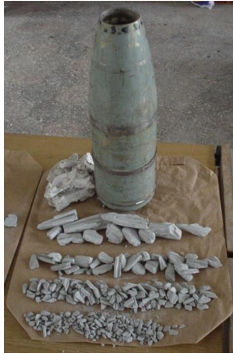
Fig. 10. Typical examples of washed out explosives fractions
