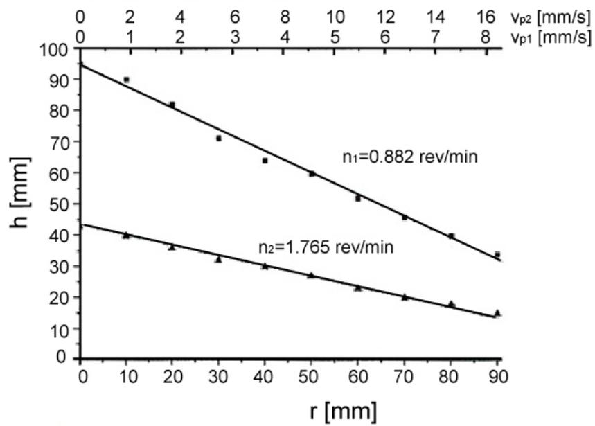
Fig. 7. Influence of the shells rotary velocity ( $n$ ) and spiral radius ( $r$ ) on the feed rate ( $v_p$ ) and explosives cut depth ( $h$ ) defined during spiral tests.
