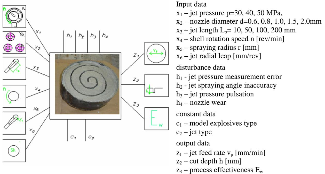
Fig. 3. General schema of research object including explosives erosion process optimization
