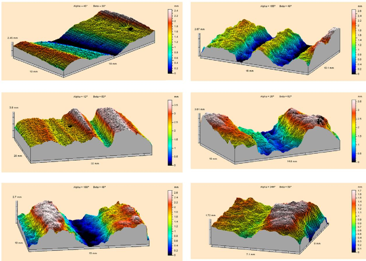
Fig. 13. Exemplary morphology scans of washed out explosive materials
