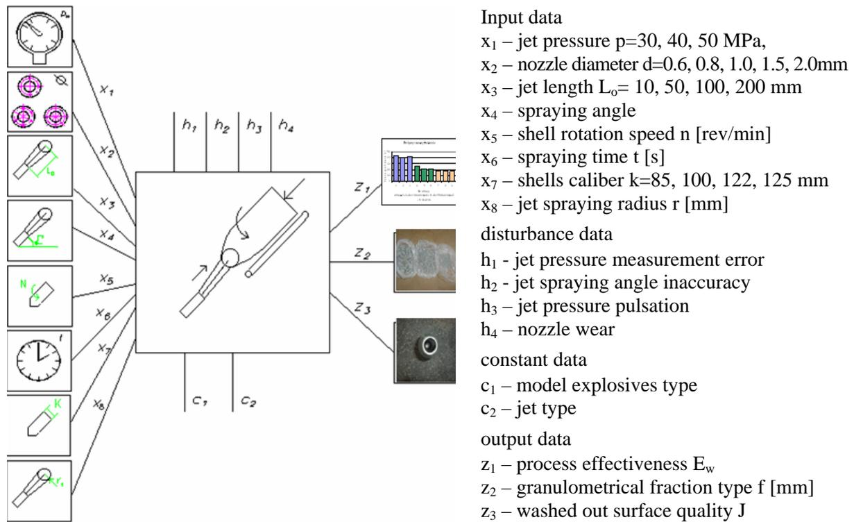
Fig. 4. General schema of research object including HPWJ shells washing out process effectiveness
