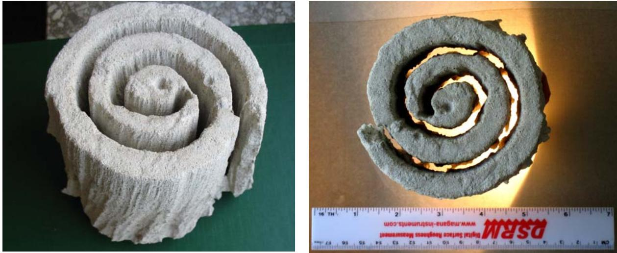
Fig. 8. Examples of explosive material washed out from artillery shells
