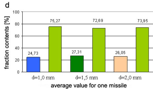
Fig. 11. Percentage contents of explosive material granulometric fractions washed out from shell cal. 100 mm ( $p=50$  MPa,  $L_0=50$  mm) using following nozzle diameters:  $d=1,0$  mm (a),  $d=1,5$  mm (b),  $d=2,0$  mm (c) and comparison of grain and sludge fraction washed out from shell (d)
