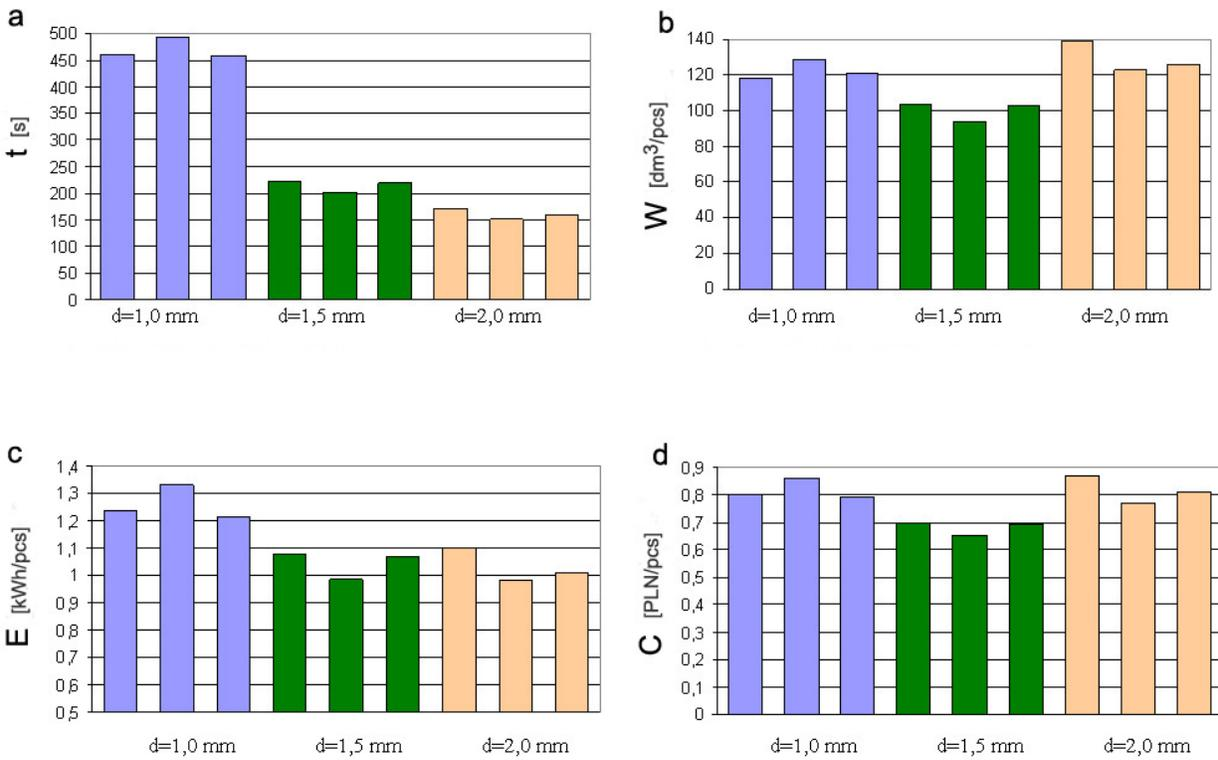
Fig. 9. Different washing out process rates indicated for shell cal. 100 mm and different nozzle types,  $p=50$  MPa,  $L_0=50$  mm. (a – time, b – effectiveness, c – energy consumption, d - costs)
